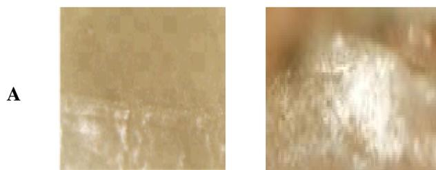
**Figure 9: A, Cohesive failure mode showing acrylic teeth remnants on base side. B. Cohesive failure mode showing porcelain remnants on base side.**
