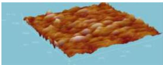
**Figure (3) Shows AFM of Sample for silicon wafer n-type (1 0 0) and resistivity of ( $\rho=10 \Omega$ . cm) Using the conditions of the method are different in terms of light intensity ( $1 \times 10^5$ ) LUX and HF 40% and time (20) min.**
