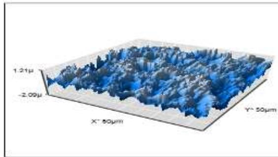
**Figure (4) Shows AFM of Sample for sample of n-type and directional silicon (1 0 0) was carried out by Electrochemical method under Current intensity ( $24 \text{ mA/cm}^2$ ) and by using 40% HF and (20) min ( $\rho= 10$ )  $\Omega$ . cm**
