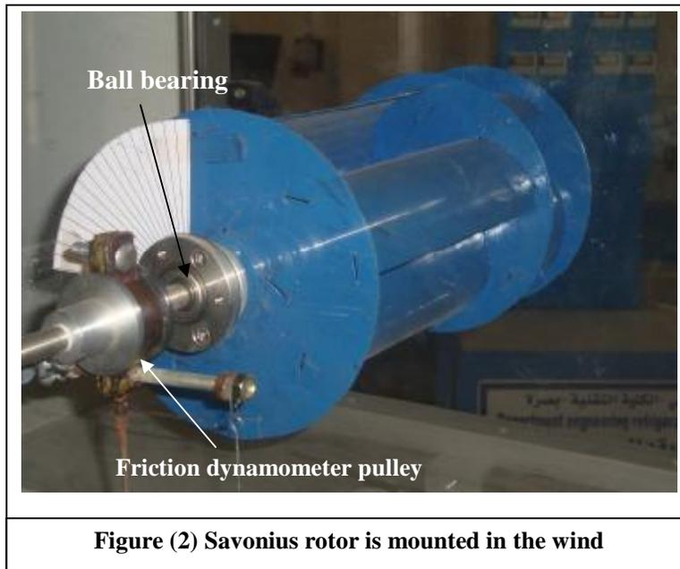
**Figure (2) Savonius rotor is mounted in the wind**
