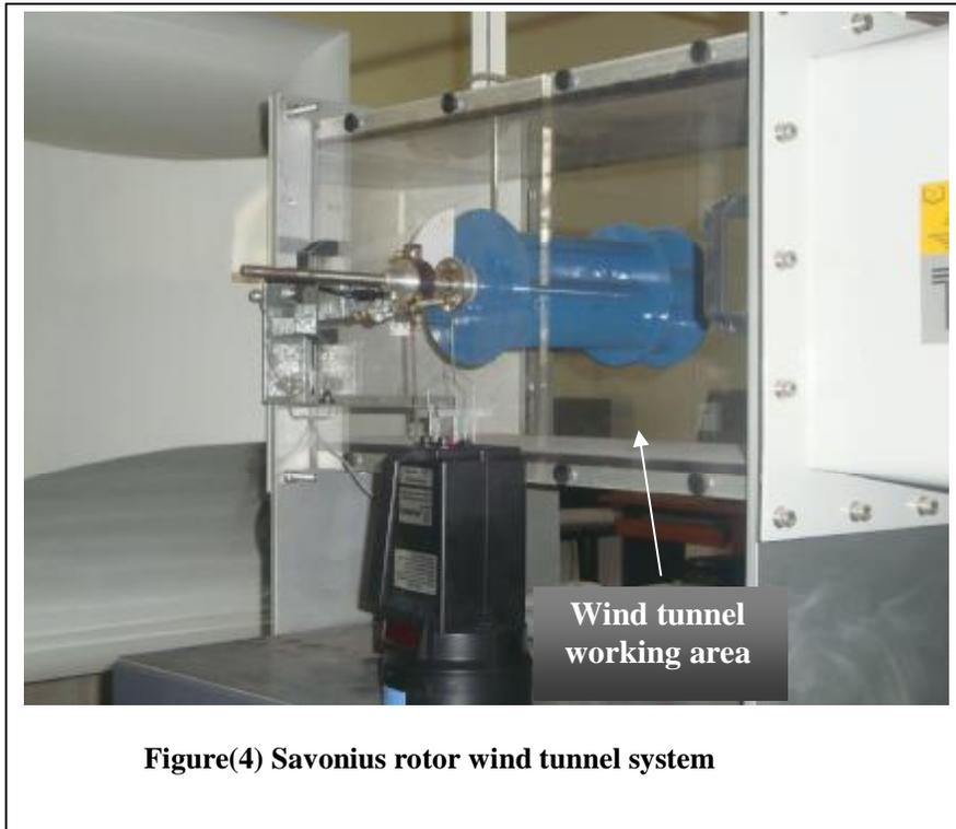
**Figure(4) Savonius rotor wind tunnel system**
