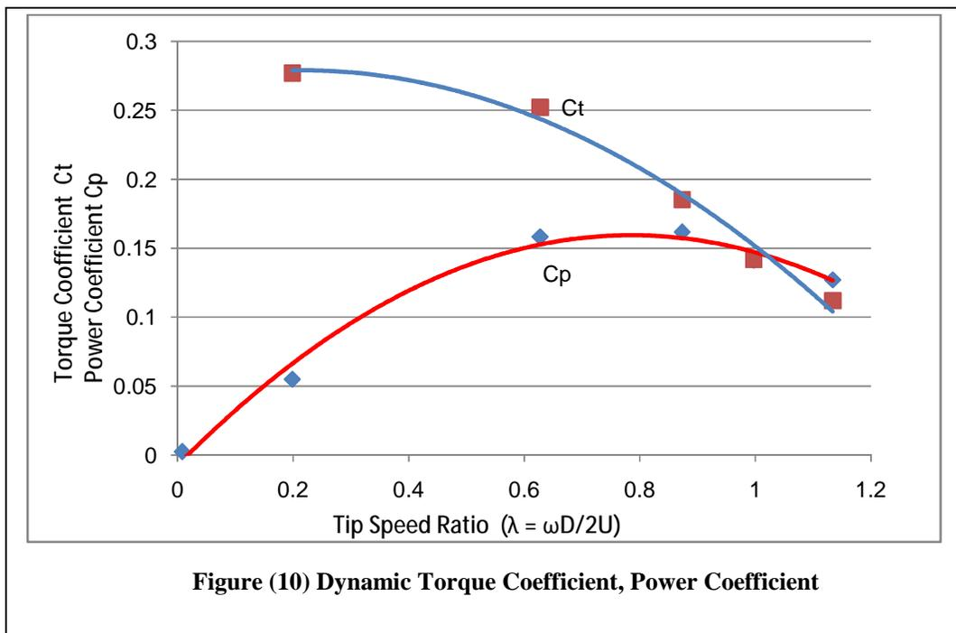
**Figure (10) Dynamic Torque Coefficient, Power Coefficient**
