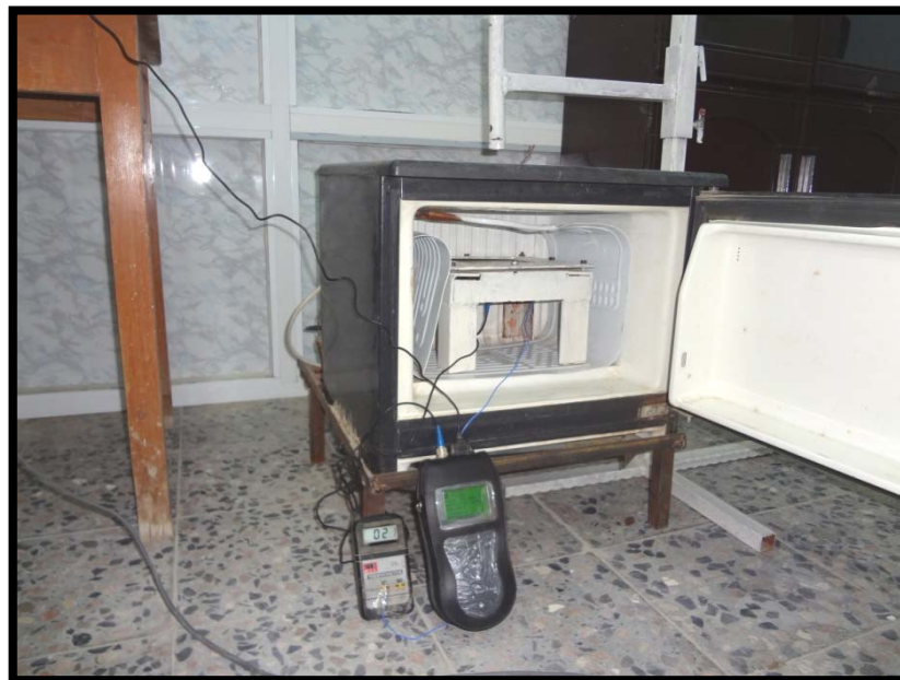
Fig. 10 : Fixed Support frame inside the refrigerating device.
