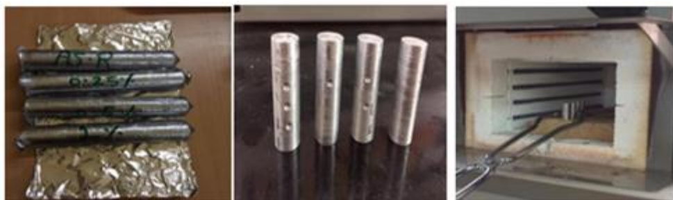
Fig. (1) The alloy specimens with difference weight percentage after preparation and heat treatment in RWF rapid wire chamber furnaces.
