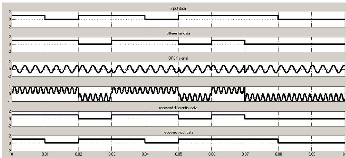
Figure 2 : DPSK waveforms
