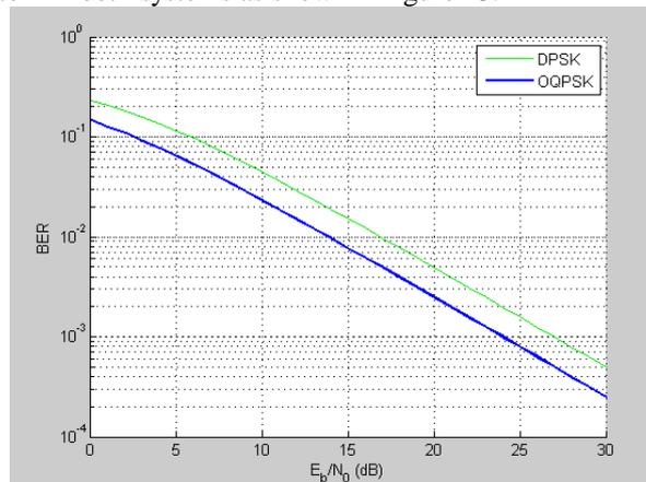
Figure 11: DPSK and OQPSK in Rayleigh fading channel
