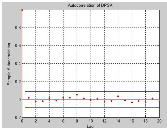
Figure 5 : auto correlation of DPSK signal
