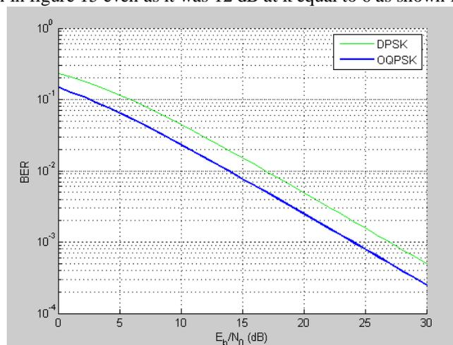
Figure 14: DPSK and OQPSK in Rician fading channel
