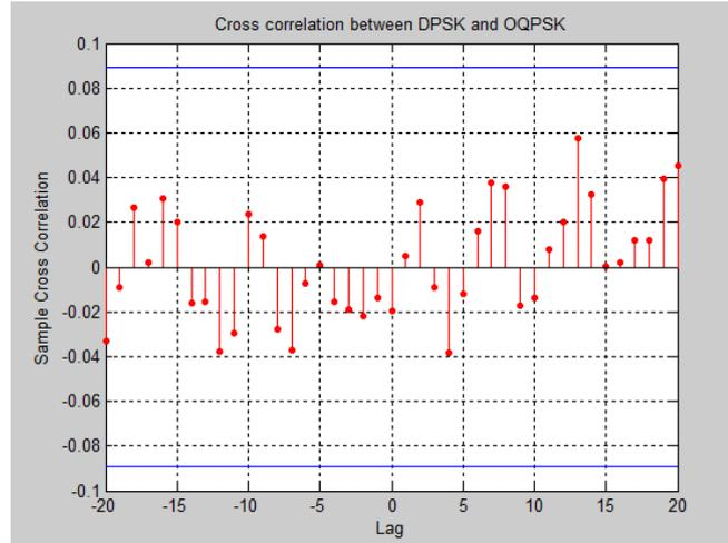
Figure 7: Cross correlation between DPSK and OQPSK signals
