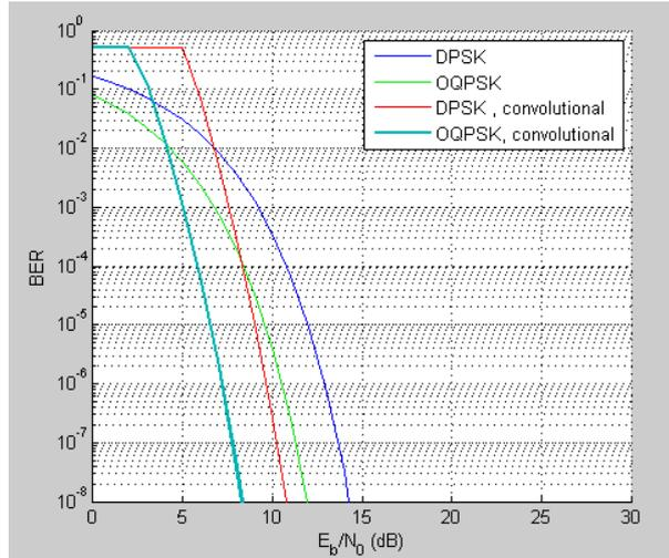
Figure 9: DPSK and OQPSK in AWGN with convolution code
