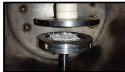
**Figure 3: PE fiber between anode and cathode.**
