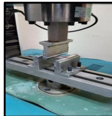
**Figure 6: Instron (examination machine for flexing test)**
