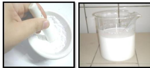
**Figure 2: Modified nanoparticles before and after dryness A: silanol containing nanoparticles; B: nanoparticles after 14 days.**
