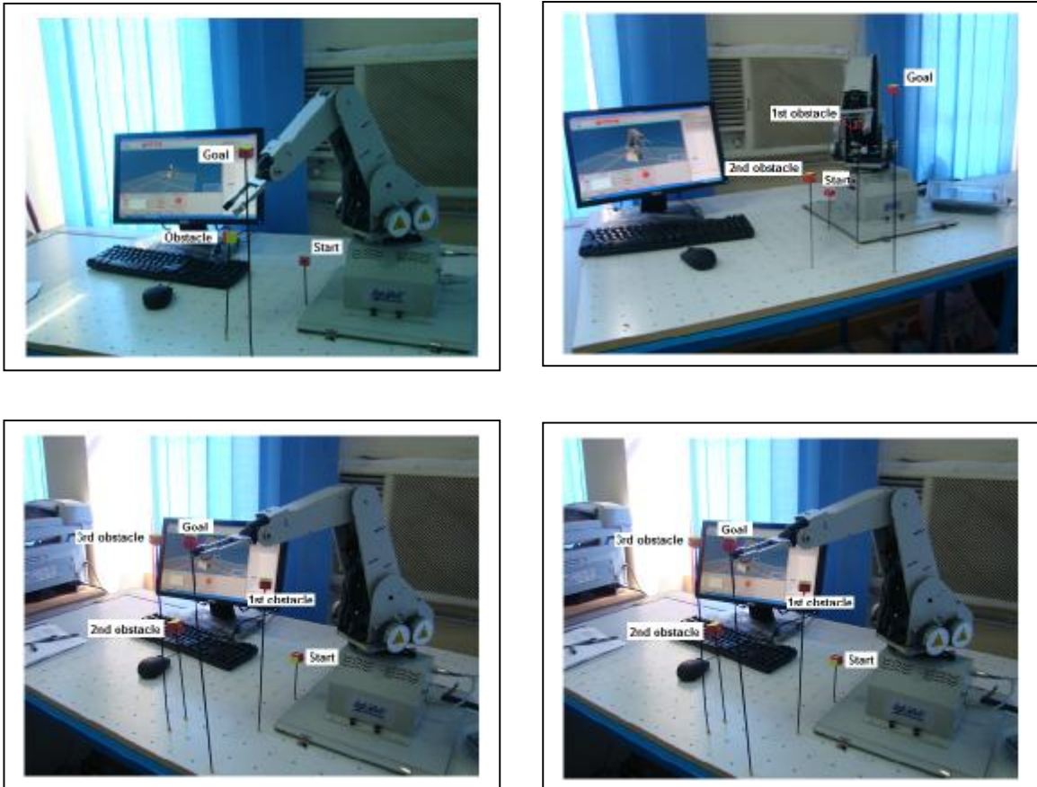
Figure (11) Testing of the LabVolt R5150 using the adopted method.
