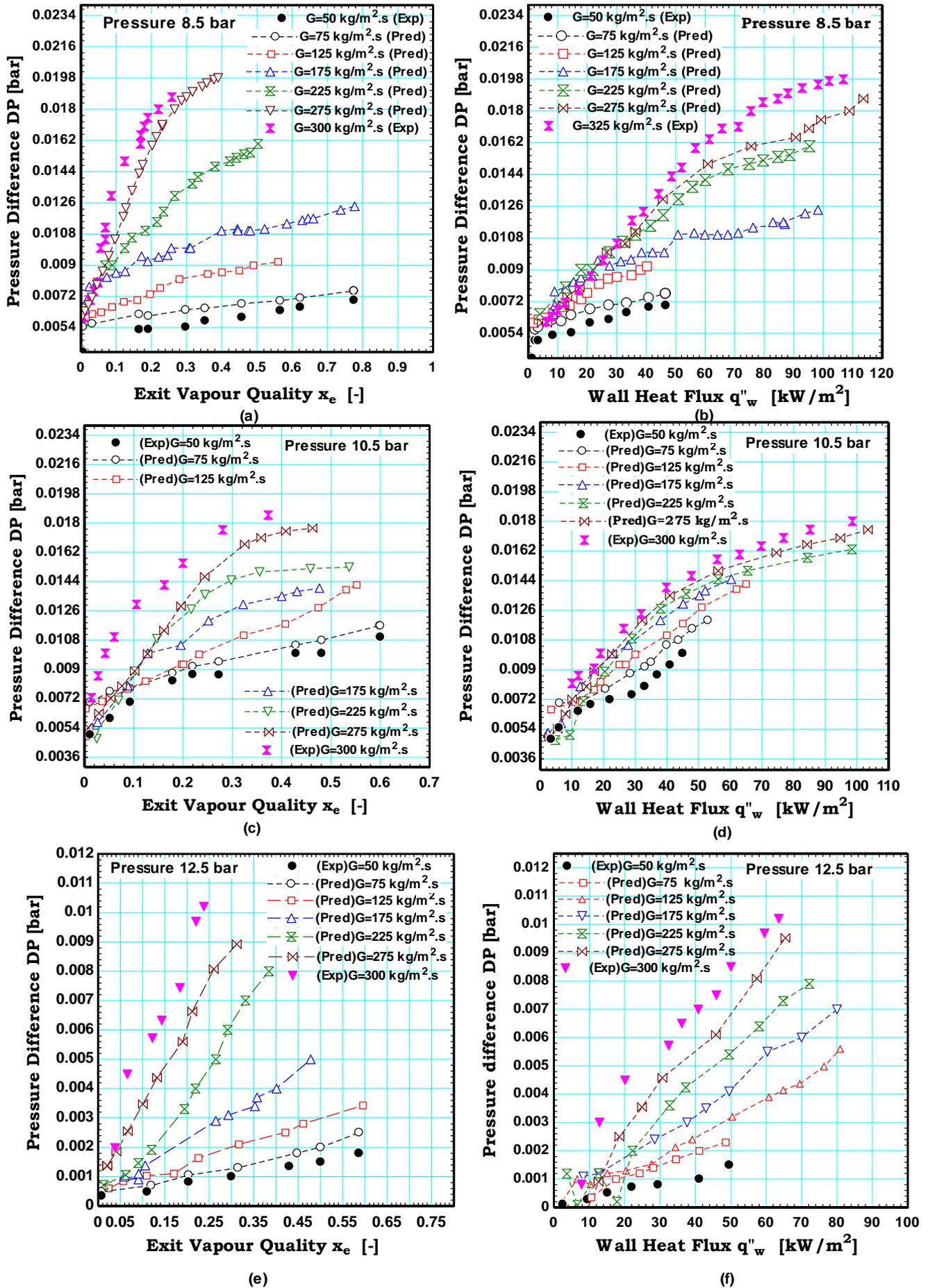
Figure 5. ANN predicted and experimental pressure drop data.
