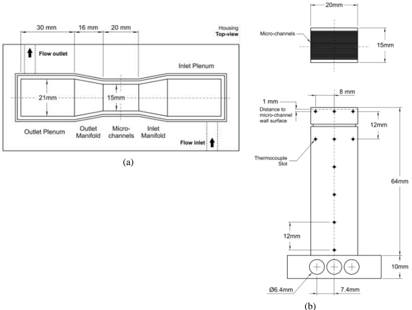
Figure 1. Schematic diagram of the test section components, (a) Housing Polycarbonate, (b) Microchannels copper part.
