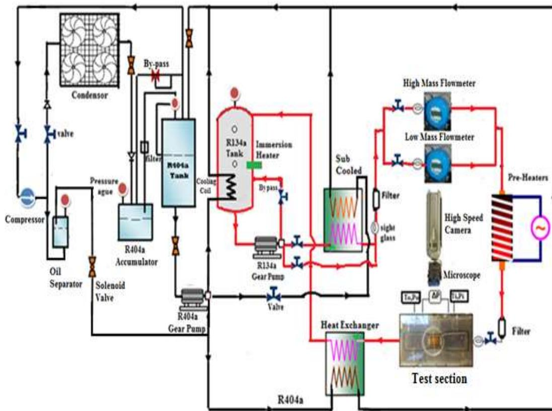
Figure 2. Schematic diagram for test loop and cooling system.
