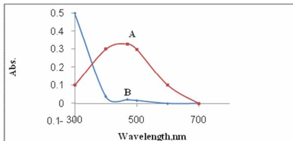
**Fig. 1: Absorption spectra of the azo dye (8 ppm) of Methyldopa against reagent blank (A) and blank against distilled water (B).**
