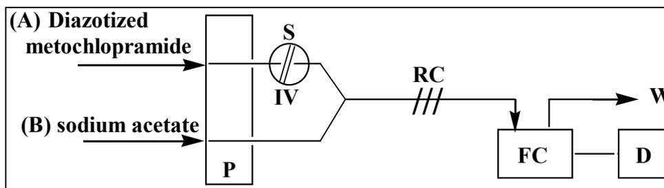
**Fig. 3:** A schematic diagram of FIA manifold Where: (A) and (B), solutions of diazotized metochlopramide and sodium acetate respectively; PP =peristaltic pump; S= injection sample Methyl dopa; IV= injection valve; T= T-link; RC= reaction coil; FC= flow cell; D= detector; W= waste.
