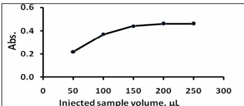
**Fig. 8: Effect of the injection loop ( $\mu\text{L}$ )**
