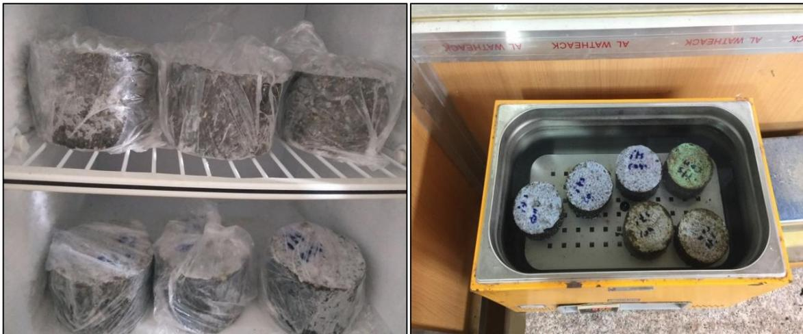
**Figure 2.** ITS test/ specimens freezing at a temperature of ( $-18\pm 3^{\circ}\text{C}$ ).
