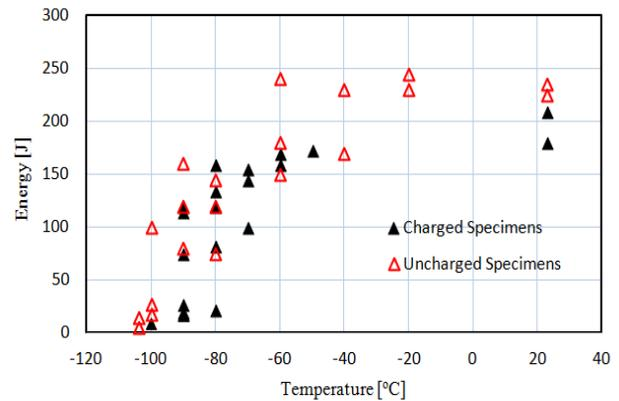
Fig. 2: Impact energy vs. temperature for X42 Steel
