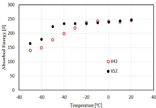
Fig. 6: Average transition curves obtained in charpy tests
