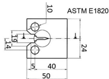
Fig.1: Specimen geometry (Note: all dimensions)
