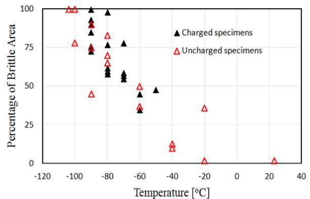
Fig. 3: Percentage of brittle area vs. temperature for X42
