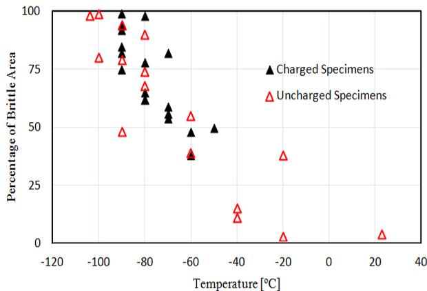
Fig. 5: Percentage of brittle area vs. temperature for X52
