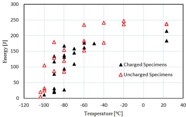
Fig. 4: Impact energy vs. temperature for X52 Steel
