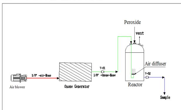
Figure 2. Schematic diagram of the H<sub>2</sub>O<sub>2</sub>/ozone system
