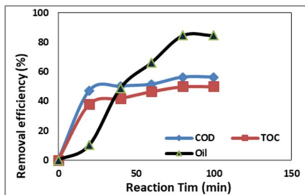
Figure 3. Effect of reaction time on removal efficiency of COD, TOC, and oil using H<sub>2</sub>O<sub>2</sub>/UV process.
