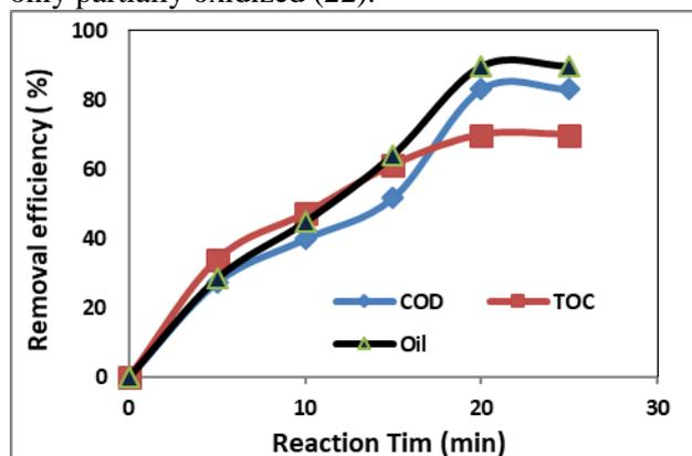
**Figure 5** Effect of reaction time on removal efficiency of COD, TOC, and oil using O<sub>3</sub>/H<sub>2</sub>O<sub>2</sub> process.
