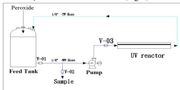
Figure 1. Schematic diagram of the  $H_2O_2/UV$  system
