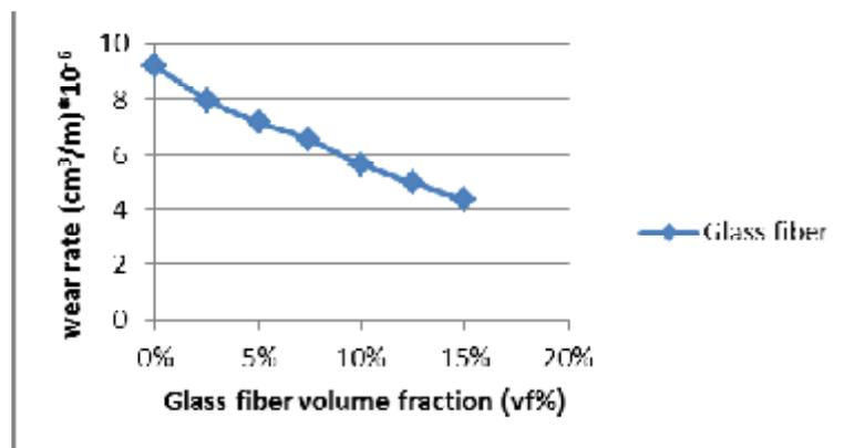
**Fig (4) Effect of volume fraction on wear rate of glass fiber.**
