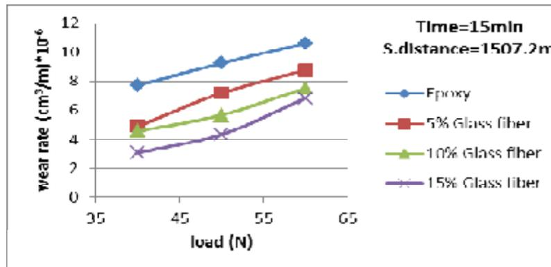
**Fig (6) Effect of load on wear rate of glass fiber.**
