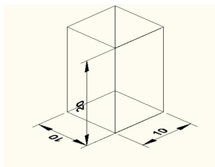
Fig (2) Standard wear test specimen.
