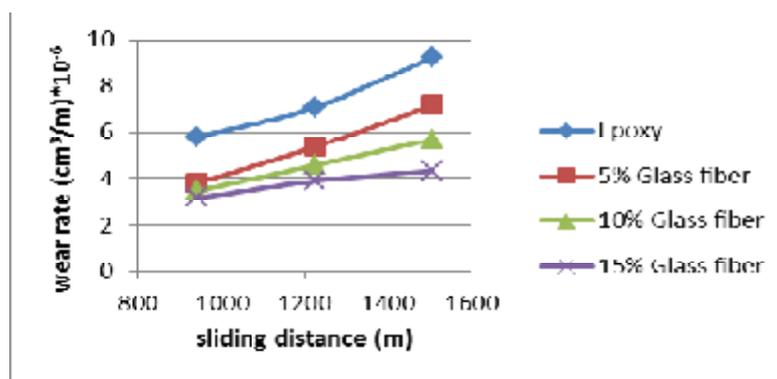
**Fig.(10) Effect of sliding distance on wear rate of glass fiber.**
