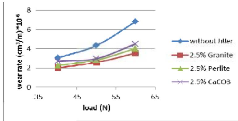
Fig.(7) Effect of load on wear rate of granite, perlite, CaCO<sub>3</sub> with 15% glass fiber.
