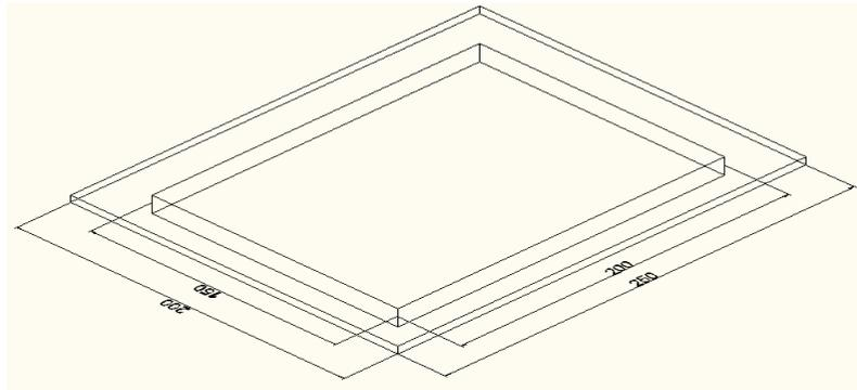
Fig (1) The shape of the mould.
