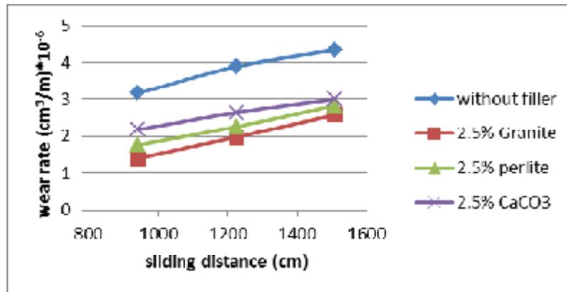
**Fig.(11) Effect of sliding distance on wear rate of granite, perlite, CaCO<sub>3</sub> powder with 15% glass fiber.**
