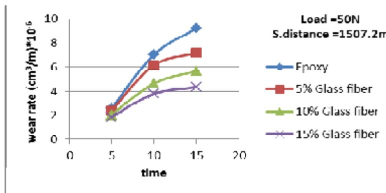
Fig. (8) Effect of time on wear rate for glass fiber.
