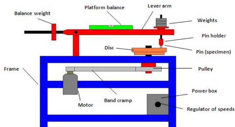
Fig (3) Schematic of pin-on-disc wear testing machine.
