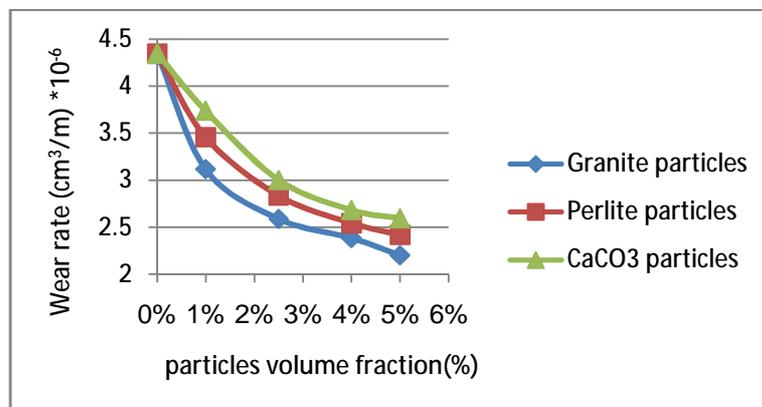
**Fig (5) Effect of volume fraction on wear rate of granite, perlite, CaCO<sub>3</sub> particles with 15% glass fiber.**
