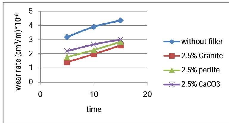
**Fig. (9) Effect of time on wear rate of granite, perlite, CaCO<sub>3</sub> powder with 15% glass fiber.**
