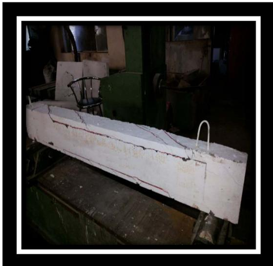
Figure (14): Crack Pattern and Failure (B2) of
