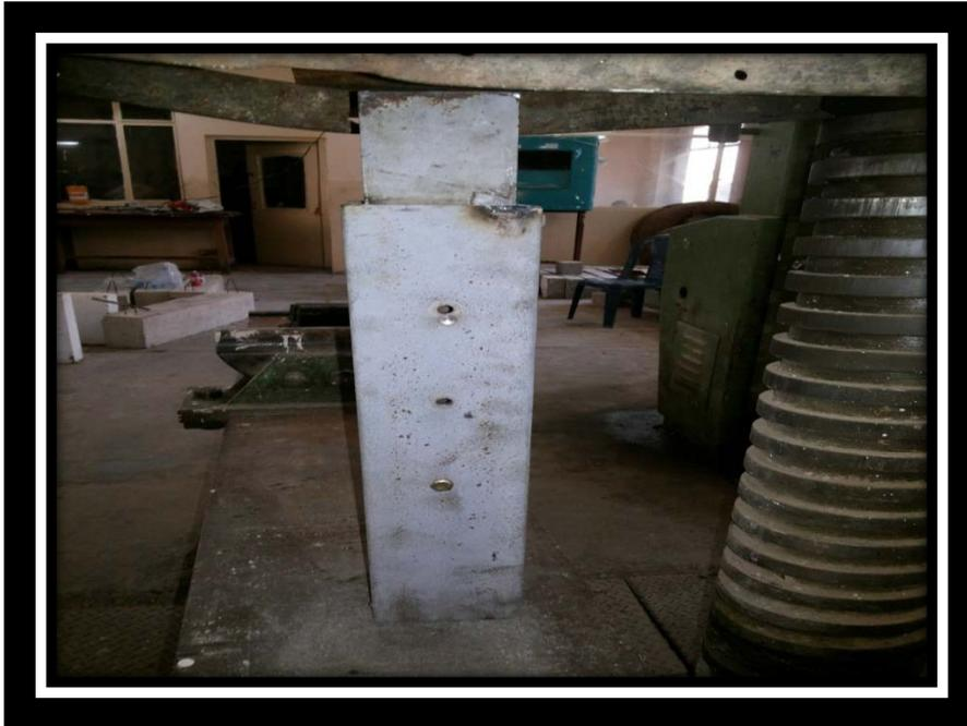
**Figure (4): Direct shear test apparatus with shear connector under testing machine.**
