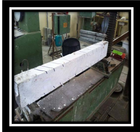
Figure (13): Crack Pattern and Failure
