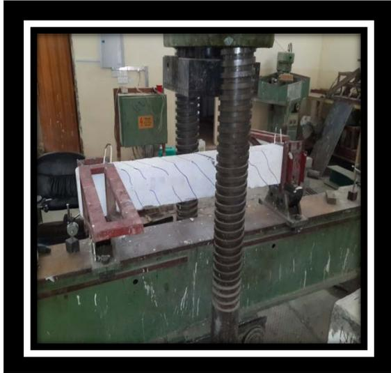
Figure (12): Failure of Reference (BN)
