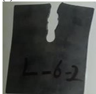
Fig (4) Tear-out Failure
