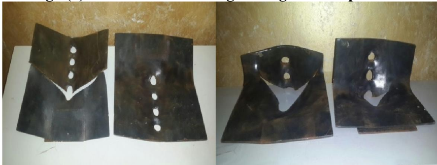
Fig. (6) Out-of Plane Curling and Diagonal Tears
