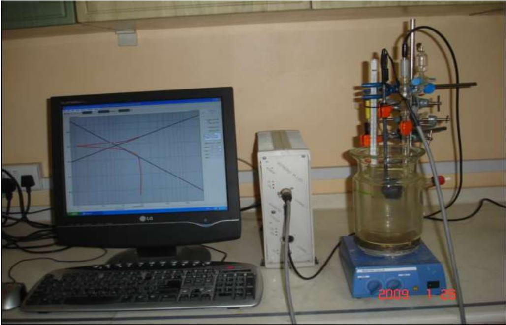
Fig. 6 The electrochemical corrosion unit and its cell.
