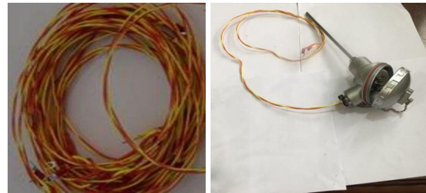
a- Thermocouple used for steel. b- Thermocouple used for concrete.
