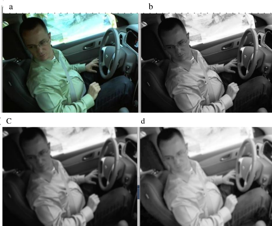
Figure 9. Samples of distracted driver images after applying pre-processing steps. (a): The original image. (b) :The image after converting to grayscale. C: The image after applying a Gaussian filter. (d): The image after applying histogram equalization.
