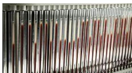
**Figure 4.** Westergren pipet array on StaRRsed automated ESR analyzer
