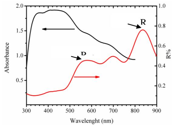
**Figure 4: Optical absorbance and reflection of porous CdS nanocrystalline thin film prepared onto FTO/glass substrate**
