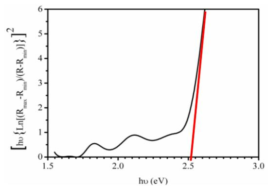
**Figure 6: Optical band gap determination of porous CdS film from reflection spectra.**
