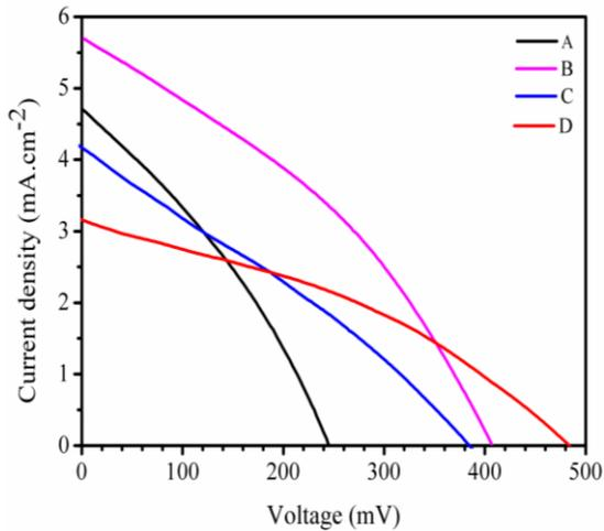
**Figure 7: J-V characteristics of the prepared DSSCs (A) porous CdS/Rhodamine B dye , (B) porous CdS/Malachite green dye, (c) porous CdS/Eosin-methylene blue dye and (D) porous CdS/Cresyl violet dye.**
