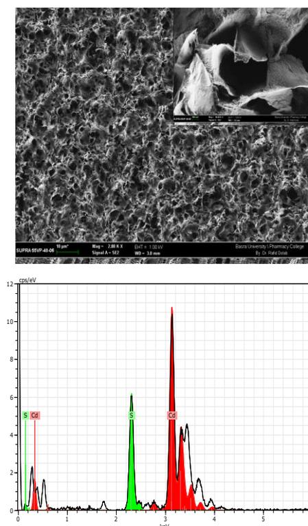
**Figure2:(A) FE-SEM micrograph of porous CdS nanocrystalline thin film, inset high magnification of thin film, (B)**
