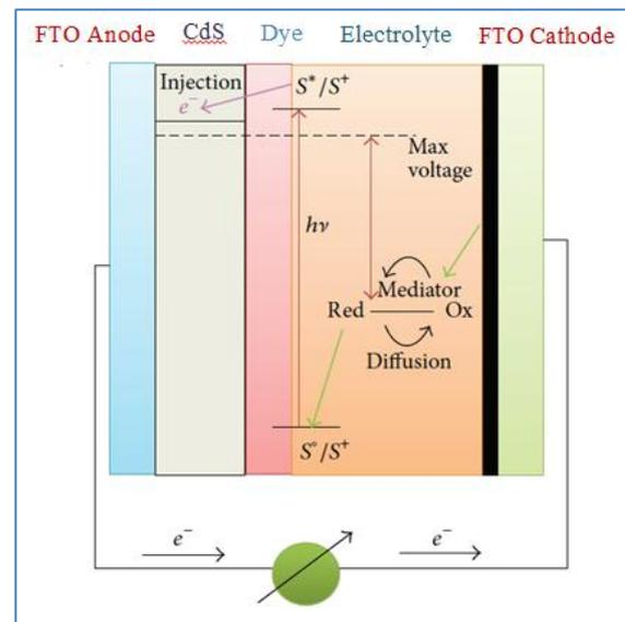
Figure 1: Structure and operating principle of dye-sensitized solar cells [24]
