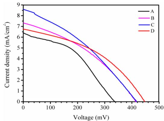
**Figure 8: J-V characteristics of prepared DSSCs after annealing process (A) porous CdS/Rhodamine B dye , (B) porous CdS/Malachite green dye, (c) porous CdS/Eosin-methylene blue dye and (D) porous CdS/Cresyl violet dye.**
