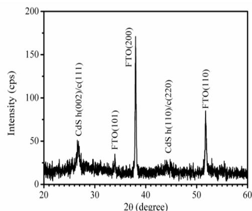
**Figure3: XRD pattern of porous CdS nanocrystalline thin film prepared onto FTO/glass substrate.**
