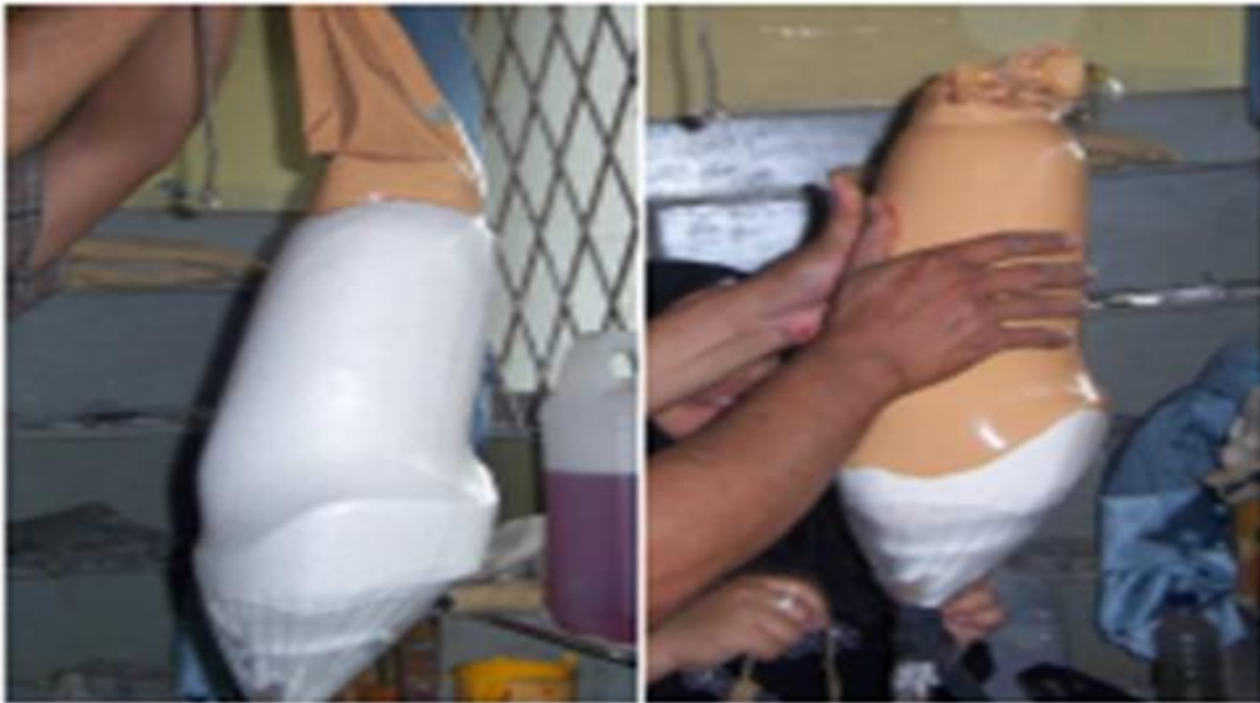
Figure 2. Socket Fabrication Procedure Using Bamboo Fiber Epoxy Composite [24].
