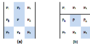
Figure (6) Examples of a ridge ending and bifurcation pixel. (a) bifurcation pixel (b) ending pixel
