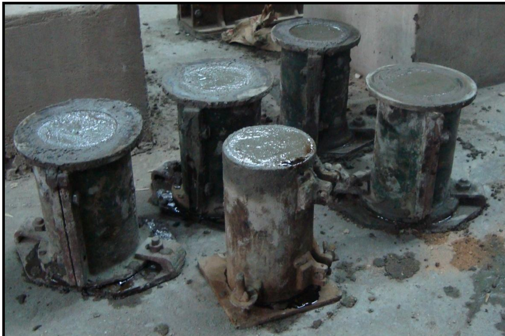
Fig. 1- Casted concrete cylinders (100*200) mm
