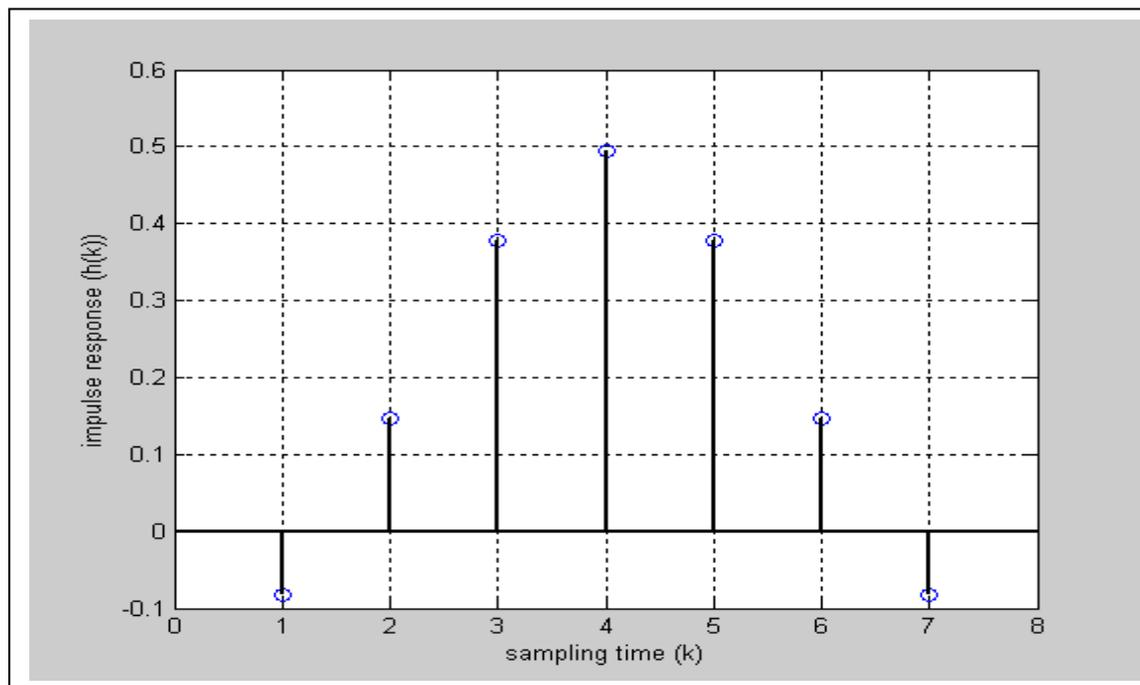
**Figure-6: Impulse response for the identified system (FIR- Low pass filter)**
