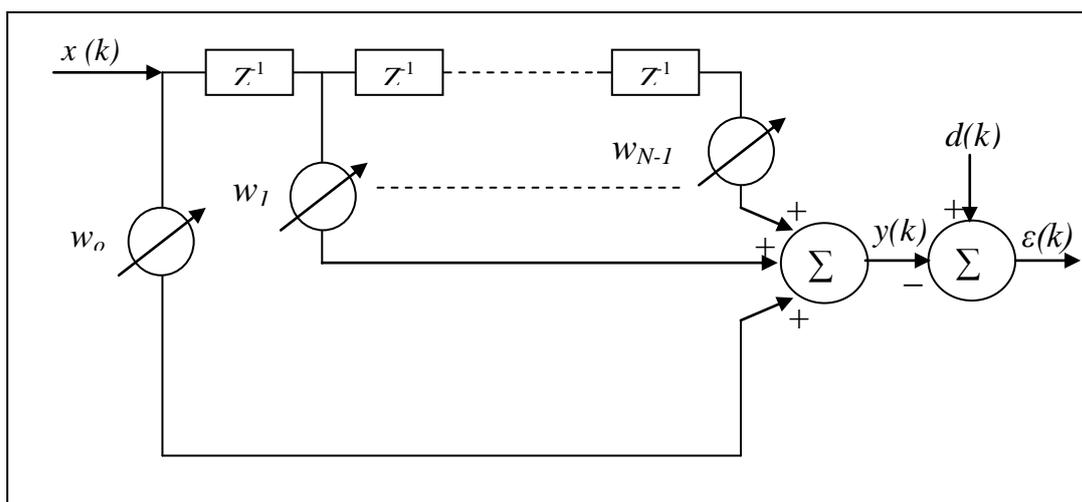
**Figure-3: The adaptive linear filter implementation**
