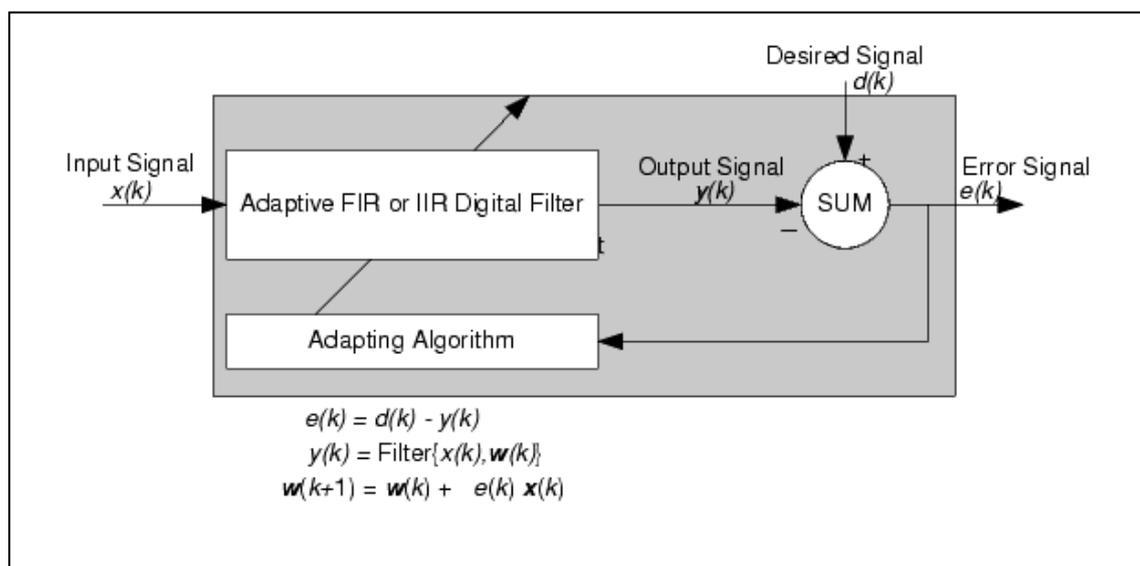
**Figure-1: Block Diagram Defining General Adaptive Filter Algorithm Inputs and Outputs**
