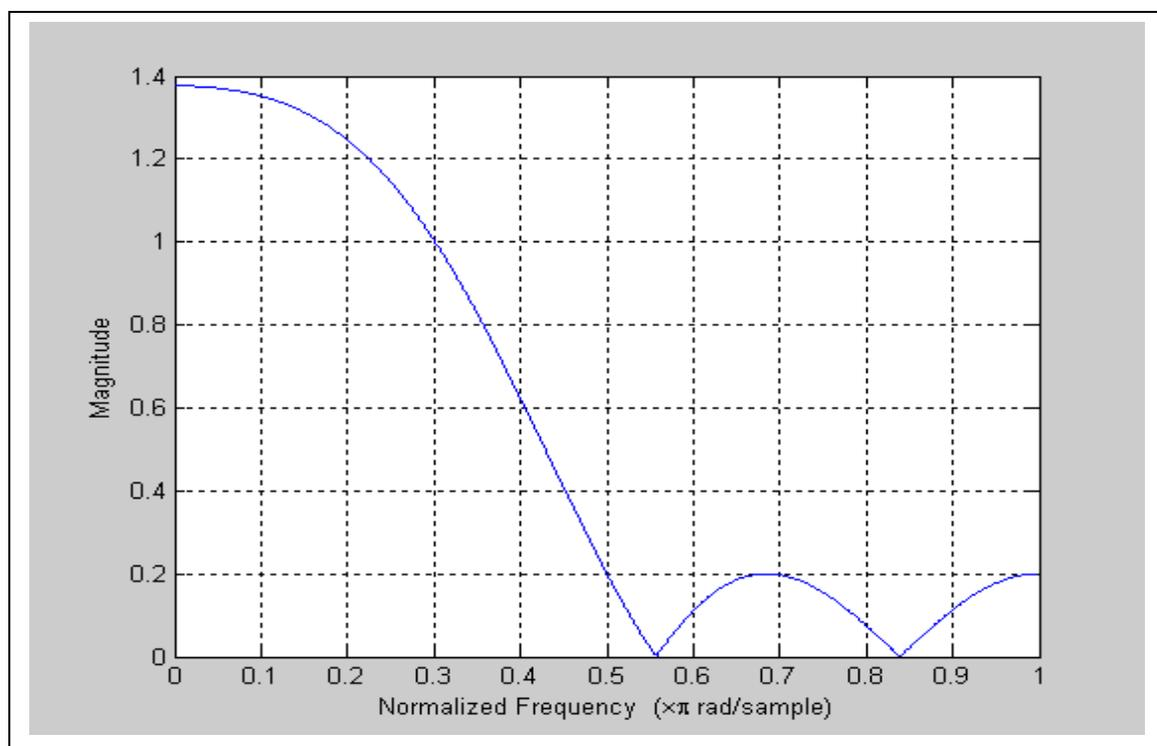
**Figure-5: Frequency response for the identified system (FIR- Low pass filter)**
