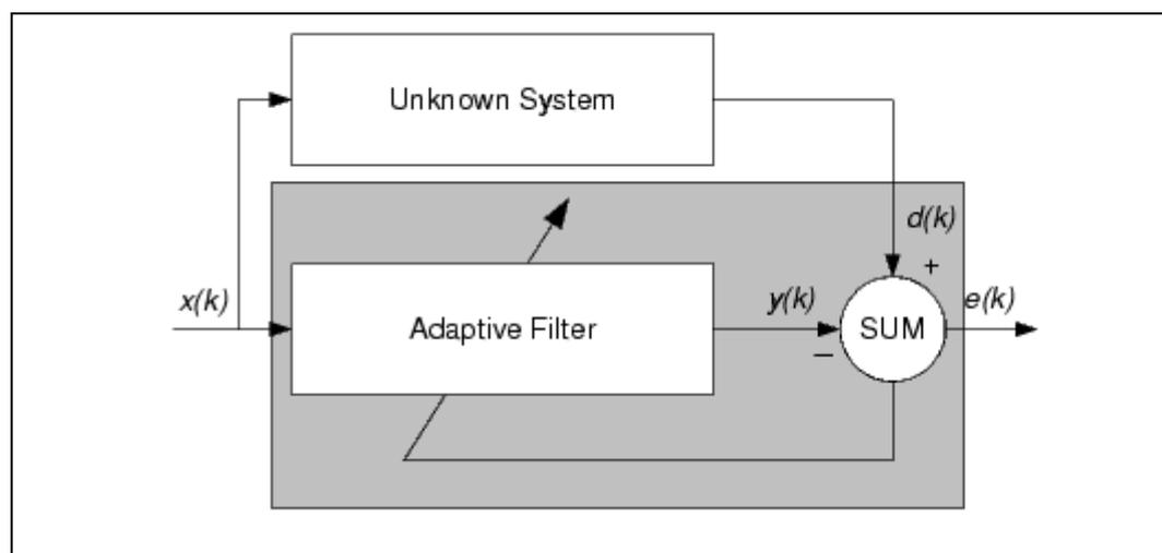
**Figure-2: Using an Adaptive Filter to Identify an Unknown System**
