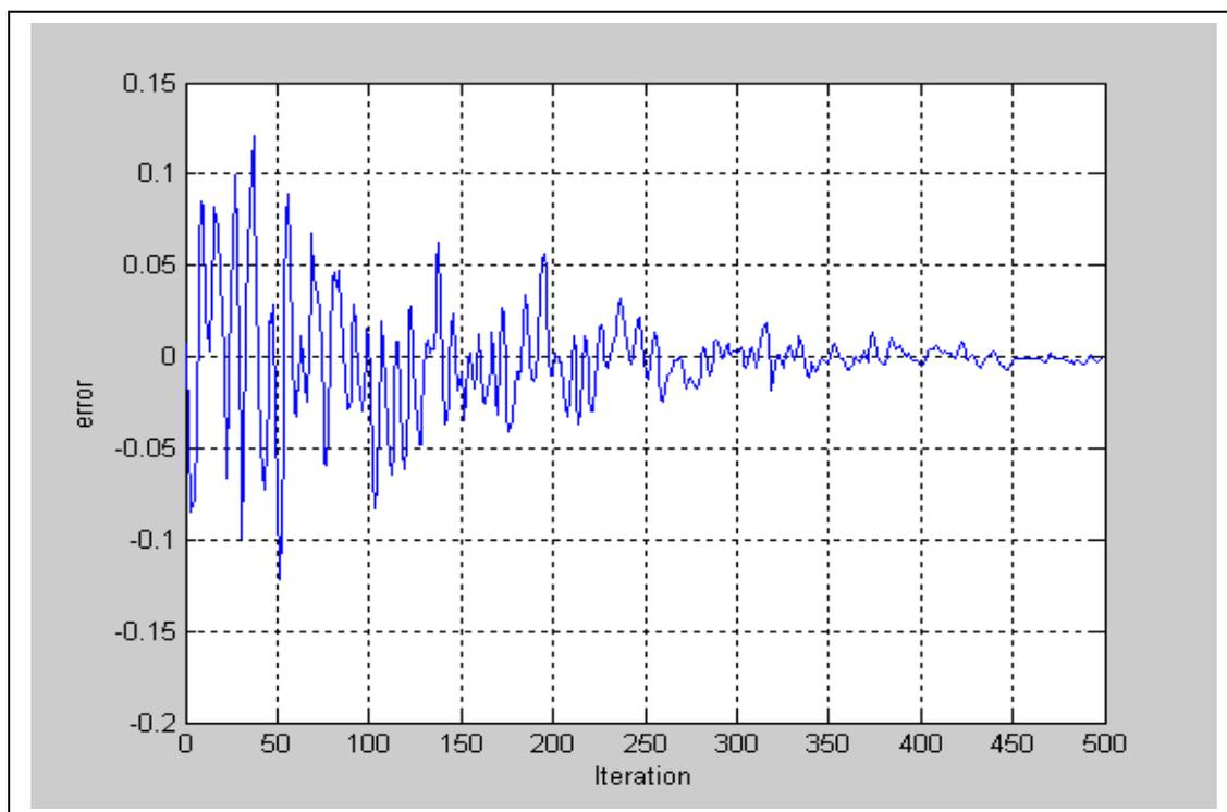
Figure-9: The learning curve for the LMS algorithm ( $\mu = 0.8$ ).
