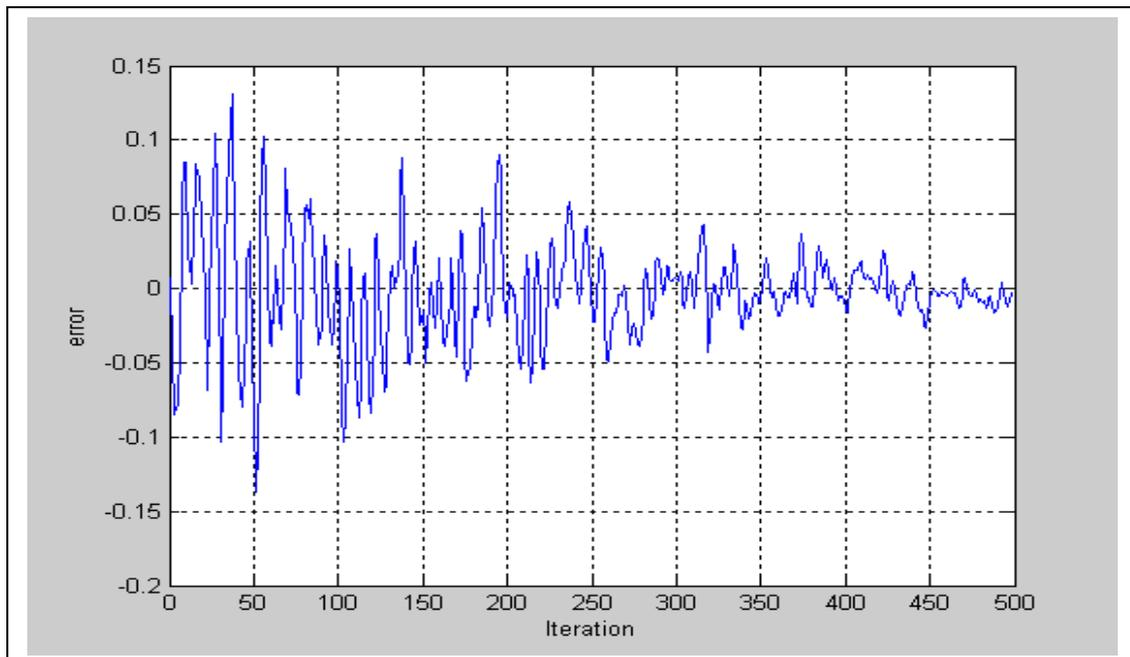
Figure-8: The learning curve for the LMS algorithm ( $\mu = 0.5$ ).
