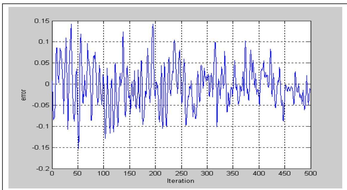
**Figure-7: The learning curve for the LMS algorithm ( $\mu = 0.2$ ).**
