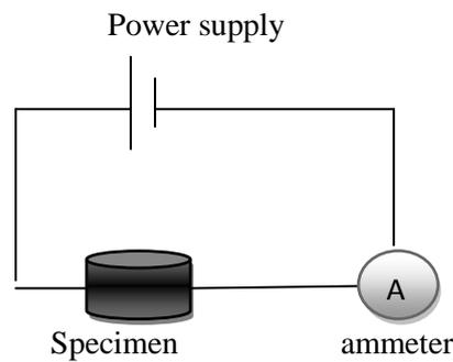
**Figure (1): schematic diagram of measurement apparatus**
