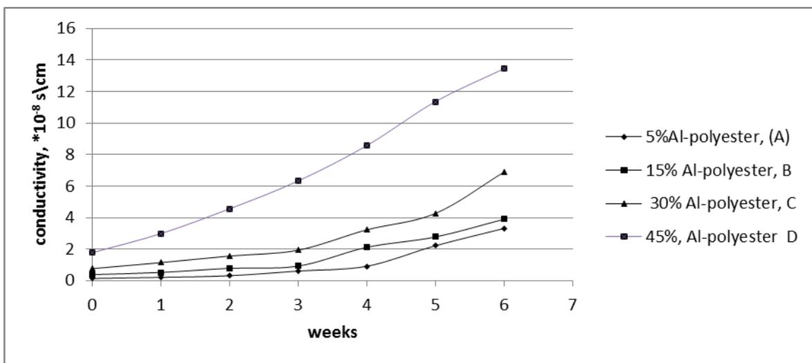
Figure (4): the variation of electrical conductivity ( $\sigma$ ) with immersed in (3.5% NaCl)
