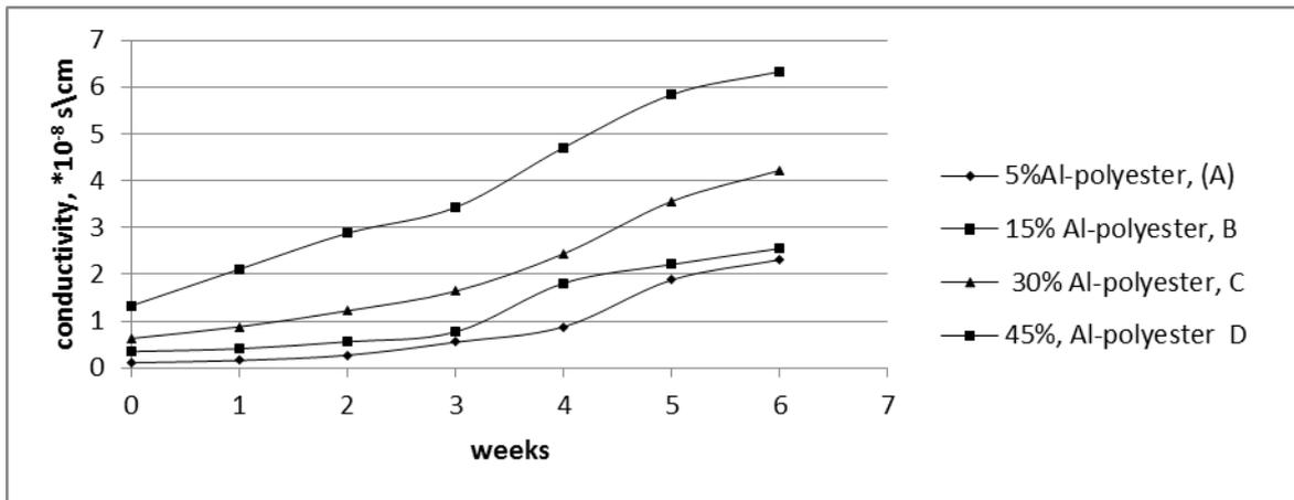
Figure (3): The variation of electrical conductivity ( $\sigma$ ) with immersed in tap water
