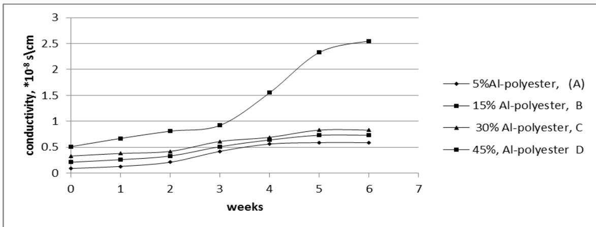
**Figure (2): the variation of electrical conductivity (σ) with immersed in distilled water**
