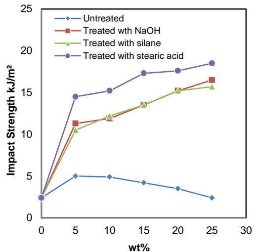
Fig. (3) The impact strength for treated and untreated eggshell powder filled UP composites with different filler loading
