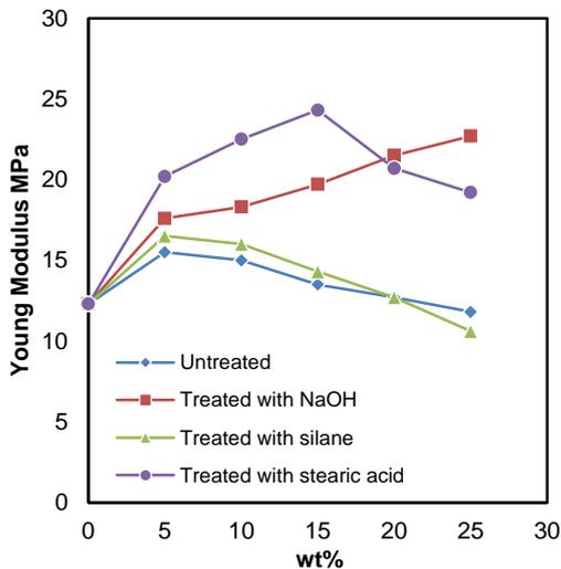
Fig. (2) The Young modulus for treated and untreated eggshell powder filled UP composites with different filler loading
