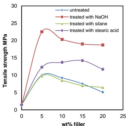
Fig. (1) The tensile strength for treated and untreated eggshell powder filled UP composites with different filler loading
