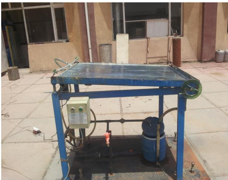
**Figure (6):** Photo-catalytic unit.
