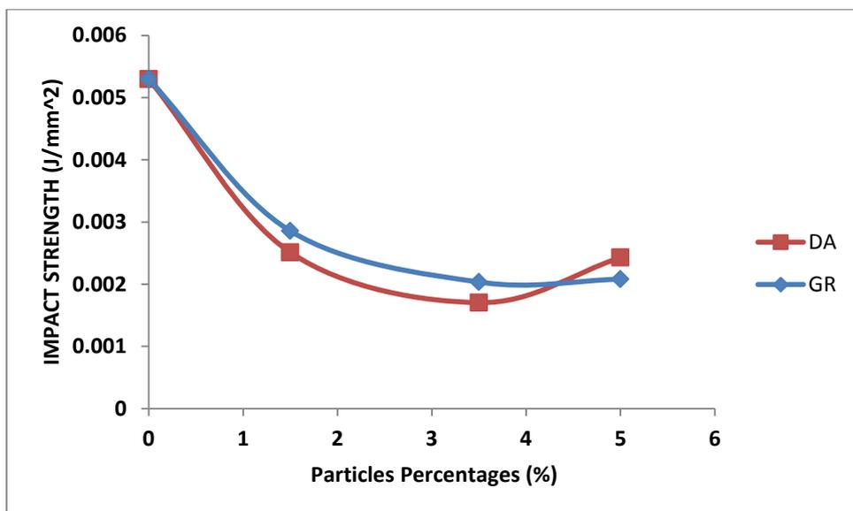
**Figure (2):** the relationship between the impact strength of unsaturated polyester reinforced with grapes and dates particles
