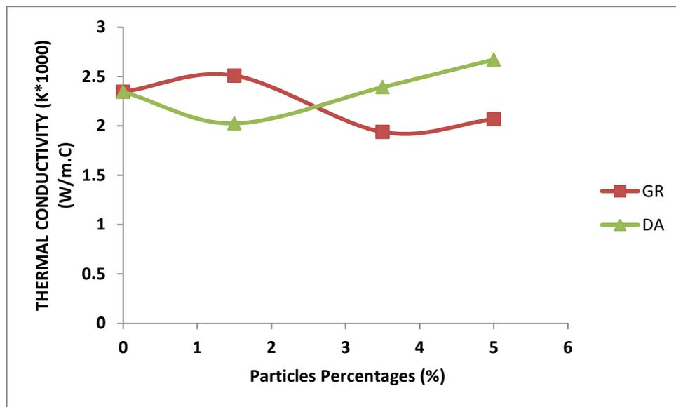
**Figure (1):** the relationship between the thermal conductivity of unsaturated polyester reinforced with grapes and dates particles
