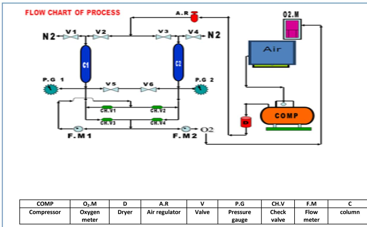
**Figure (9):** Flow diagram of PSA unit
