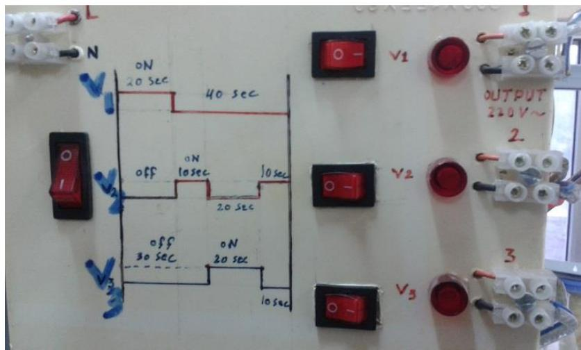
**Figure (8):** control panel 4 steps unit.
