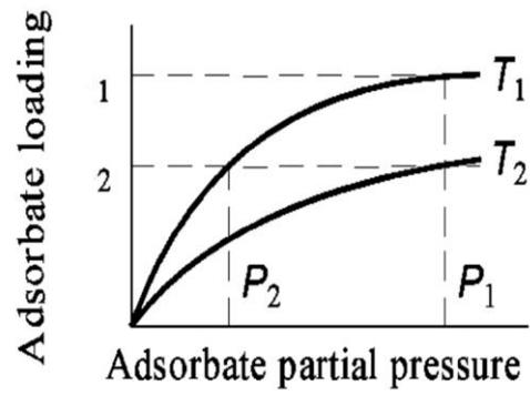
**Figure (1):** Temperature- swing and pressure-swing cycles.
