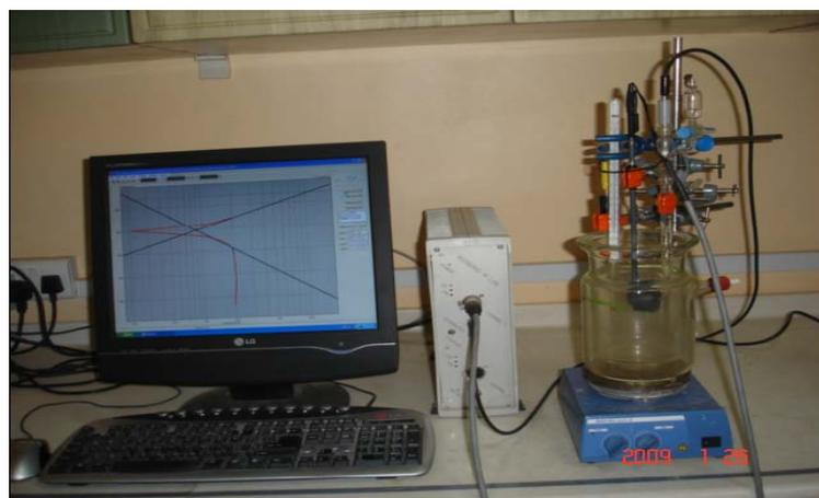
**Fig. 4** The electrochemical corrosion unit
