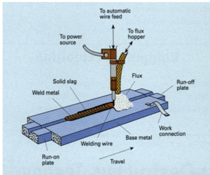
**Fig. 1** Submerged-arc Welding process
