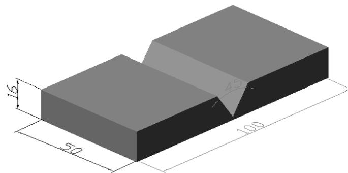
**Fig. 2** The design and dimensions of single V-butt joint
