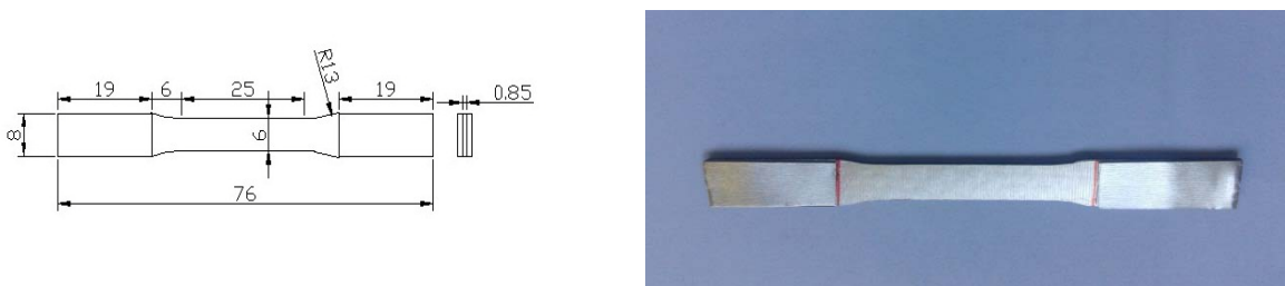
Figure (2): Tensile specimen of composite material according to ASTM D3552 (all dimensions in mm).
