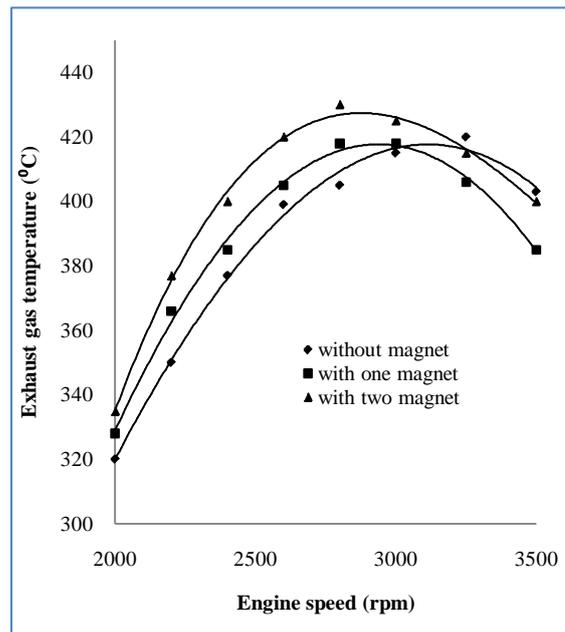
Fig. 8, Magnet effect on exhaust gas temperatures for variable engine speed
