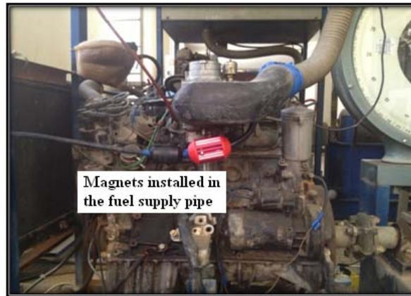
**Fig. 4, Magnets Installed in the Fuel**
