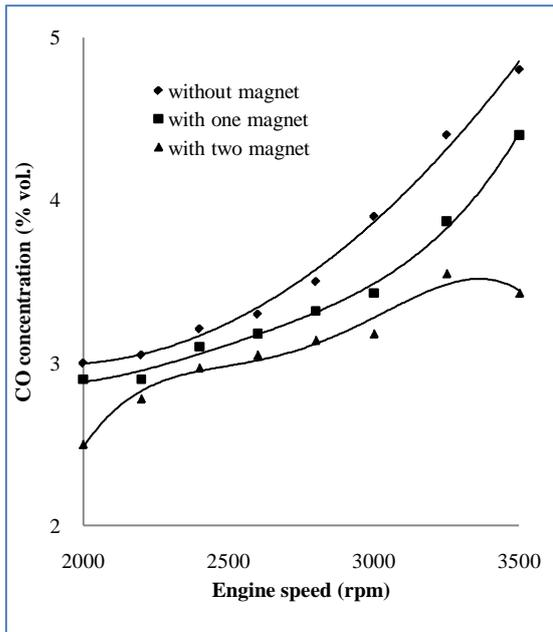
**Fig. 9, Magnet effect on CO concentrations for variable engine**
