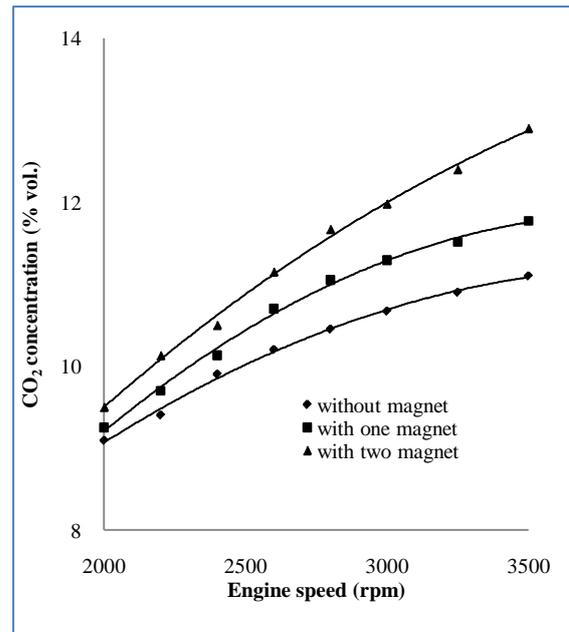
**Fig. 10, Magnet effect on CO<sub>2</sub> concentrations for variable engine speed**
