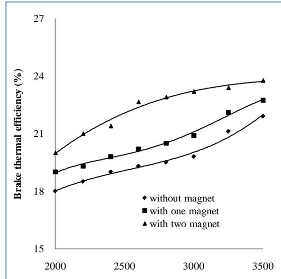
Fig. 7, Magnet effect on brake thermal efficiency for variable engine speed
