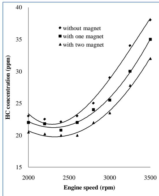
**Fig. 11, Magnet effect on HC concentrations for variable engine speed**
