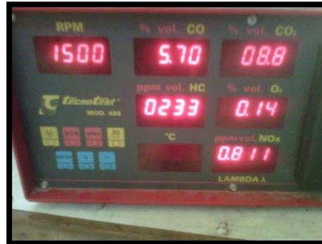
**.Fig. 2: The Exhausts Gas Analyzer Type**
