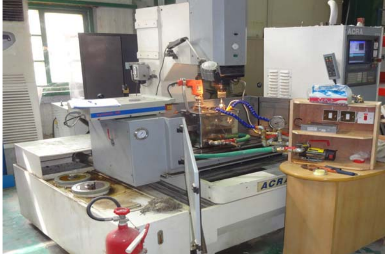
Figure(4): The (CNC) EDM machine with all the manufactured accessories designed for the implementation the PMEDM experiments
