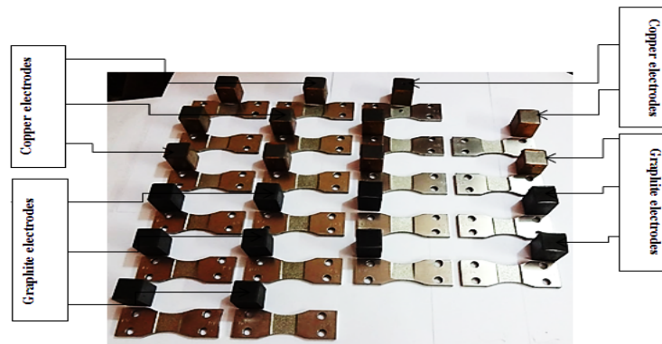
Figure (3): The copper, graphite electrodes and workpieces after PMEDM processes
