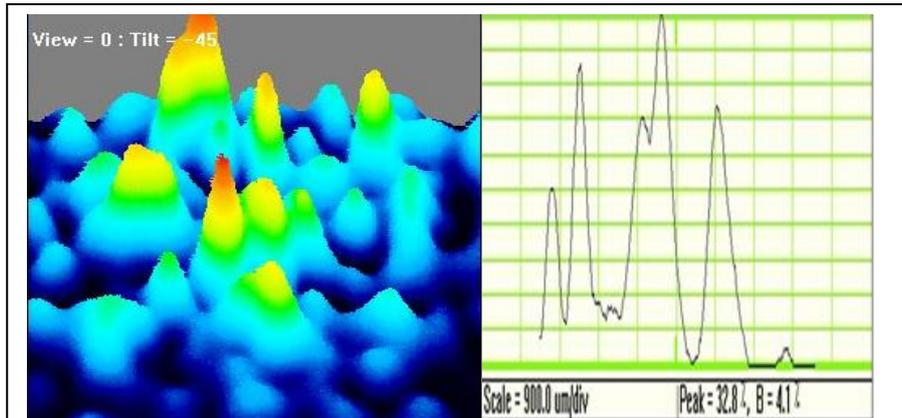
**Fig.4: Speckle pattern alarm signal in the hard vibration using CCD beam profile detector.**
