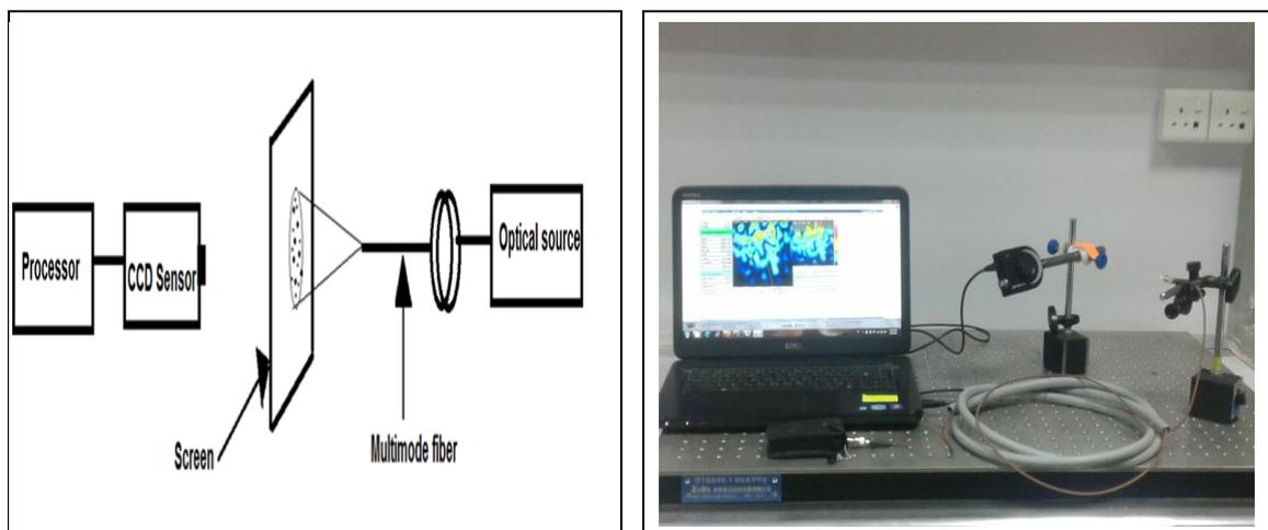
**Fig.1: The set-up of system used to record and analyze speckle patterns.**
