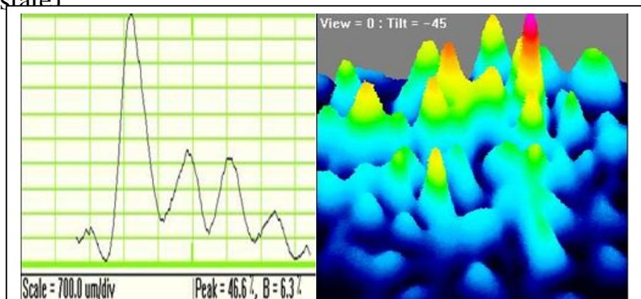
**Fig.3: Speckle pattern alarm signal in the slow intrusion using CCD beam profile detector.**
