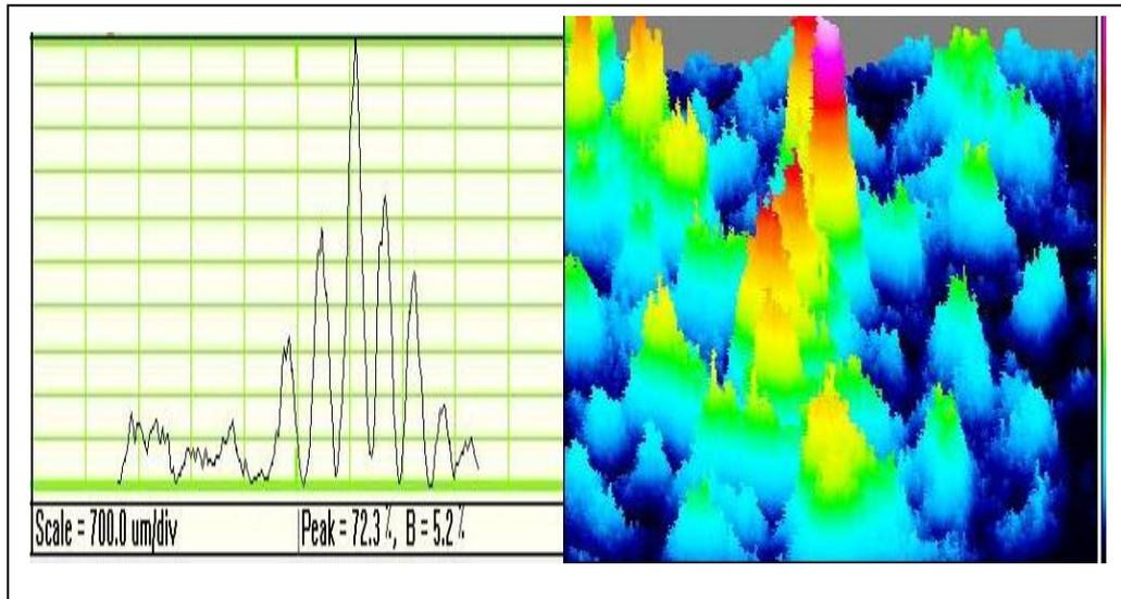
**Fig.2: Speckle pattern alarm signal in the steady state using CCD beam profile detector.**
