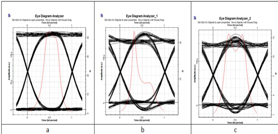
**Figure5 : Optical wireless communication of length 400km at aperture diameter 20cm (a)Eye diagram of Bessel filter (b) Eye diagram of Butterworth filter.(c) Eye diagram of Gaussian filter.**
