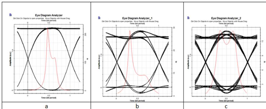
Figure8 : Optical wireless communication of length 200km at aperture diameter 30cm (a)Eye diagram of Bessel filter (b) Eye diagram of Butterworth filter.(c) Eye diagram of Gaussian filter.
