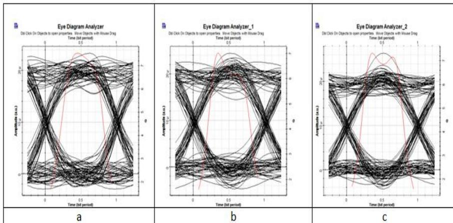
**Figure6 : Optical wireless communication of length 200km at aperture diameter 10cm (a)Eye diagram of Bessel filter (b) Eye diagram of Butterworth filter.(c) Eye diagram of Gaussian filter.**
