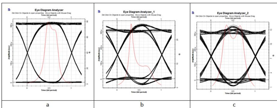
**Figure3:Optical wireless communication of length 200km at aperture diameter 20cm (a)Eye diagram of Bessel filter (b) Eye diagram of Butterworth filter.(c) Eye diagram of Gaussian filter.**
