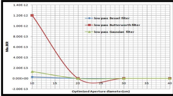
Figure 14 Min. BER. Vs, diameter for different filters
