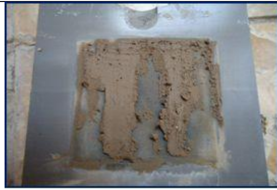
Figure 4. Concrete-Soil Interface after Failure
