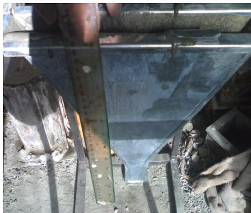
**Figure 2:** Viscosity and fillingability by V-funnel flow time test
