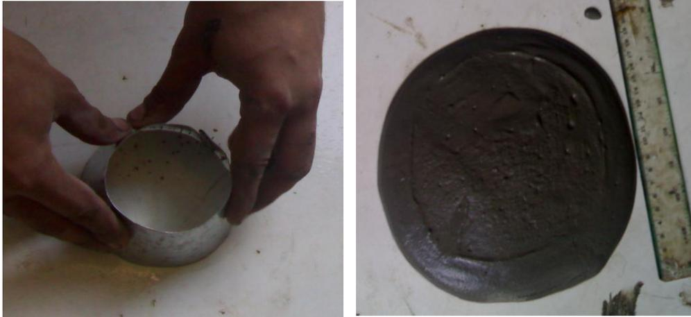
**Figure 1:** Consistency test by Flow Table
