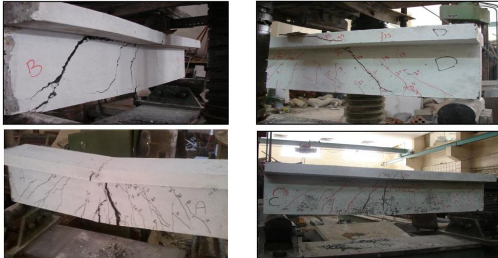
Figure 5: Crack Patterns for T-Beams
