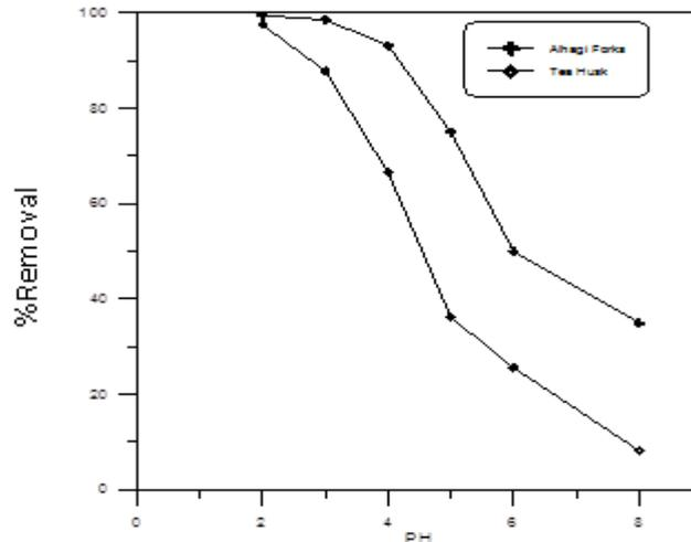
**Figure 1:** Effect of pH on Adsorption of Cr at 25oC, Weight of media 0.5g, Co of solution is 10ppm and time is 30min
