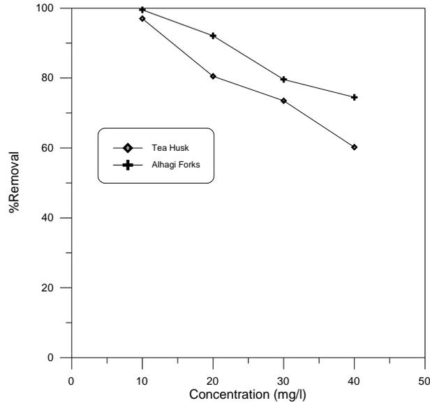
**Figure 4:** The effect of Increasing Concentration on removal of Cr(VI) ion
