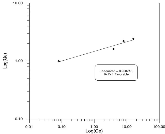
Figure 10: Freundlich Isotherm for adsorption of Cr(VI) using Alhagi Forks for 30min and pH=2
