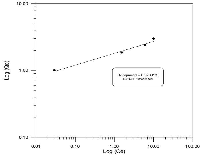
Figure 9: Freundlich Isotherm for adsorption of Cr(VI) using Tea Husk for 30min and pH=2
