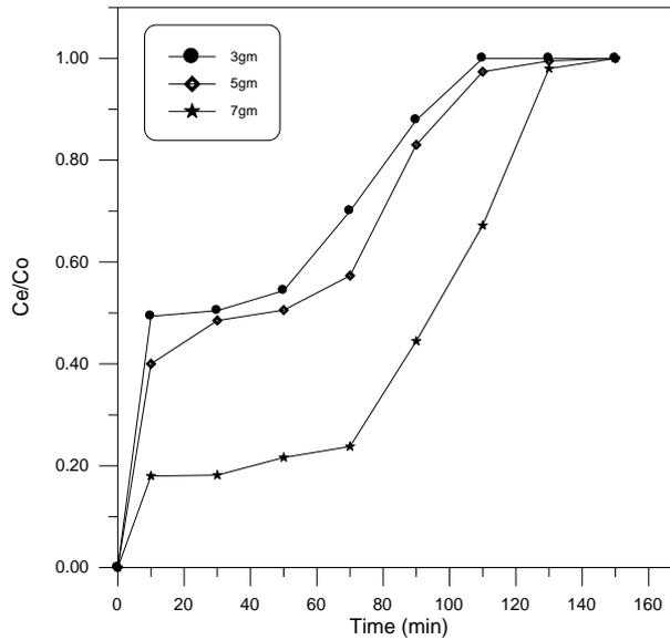
**Figure 6:** The effect of Increasing of Bed Height of Tea Husk on Breakthrough of Cr (vi) ion for 40mg/l, pH=2
