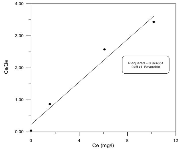
**Figure 7:** Langmuir Isotherm for adsorption of Cr(VI) using Tea Husk for 30min and pH=2
