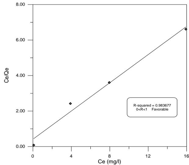
**Figure 8:** Langmuir Isotherm for adsorption of Cr(VI) using Alhagi Forks for 30min and pH=2
