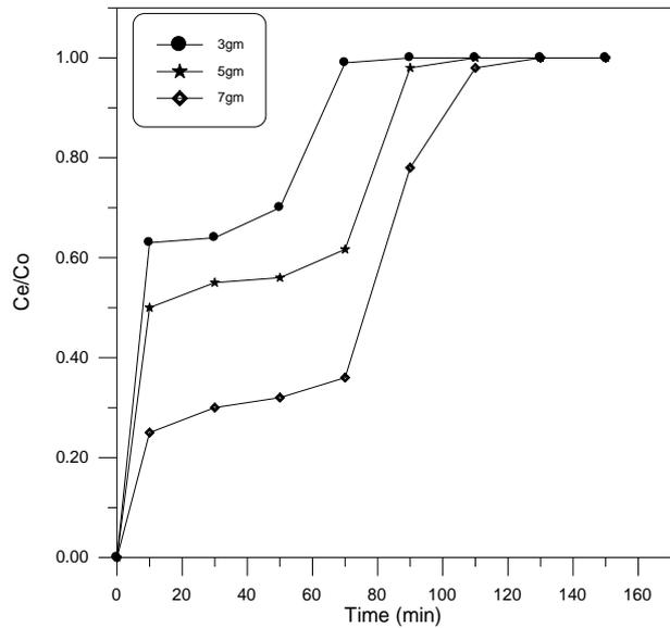
**Figure 5:** The effect of Increasing of Bed Height of Alhagi Forks on Breakthrough of Cr (vi) ion for 40mg/l, pH=2
