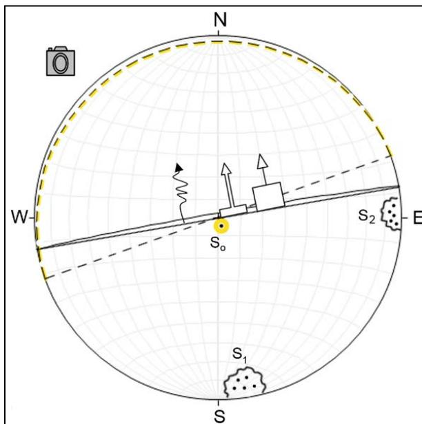
Fig.5: Stereogram of discontinuities, slope and types of failure for station No.4
