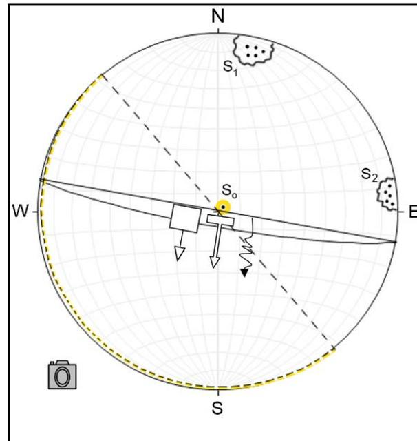
Fig.3: Stereogram of slope and types of failure for station No.2
