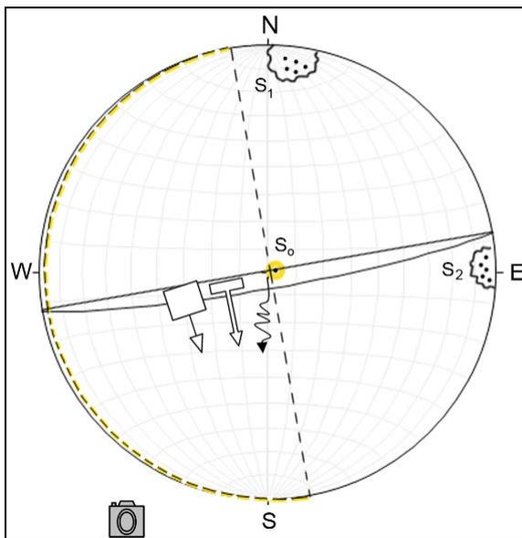
Fig.4: Stereogram of slope and types of failure for station No.3
