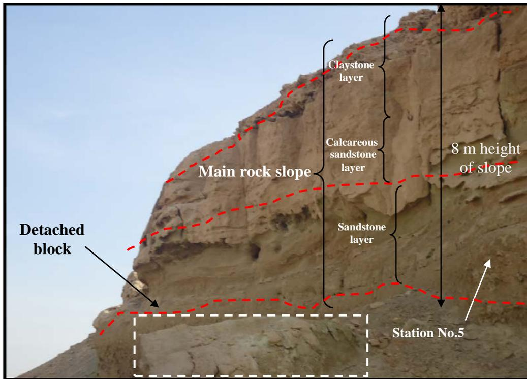
Plate 5-b: The slope of station No.5. Front view showing detached rock block and rock fall
