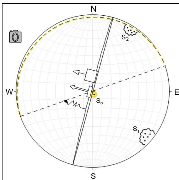
Fig.6: Stereogram of discontinuities, slope and types of failure for station No.5
