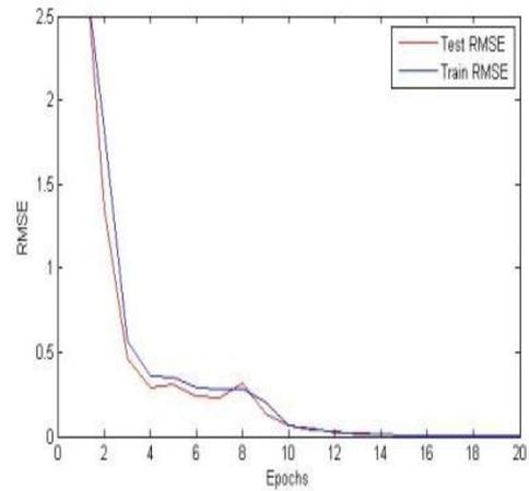
Fig.15 ANN Error Curves using Levenberg – Marquardt (trainlm)
