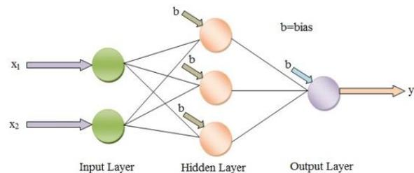
Fig.3 Basic structure of a three - layer feedforward neural network.
