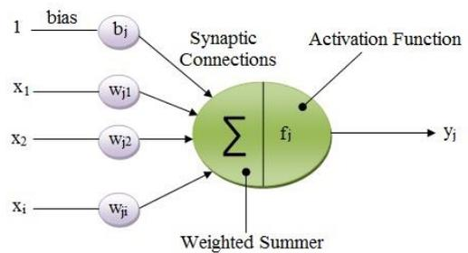
Fig.2 Basic model of a single artificial neuron.
