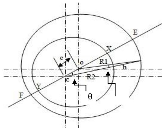
Fig.1 Section of bearing geometry
