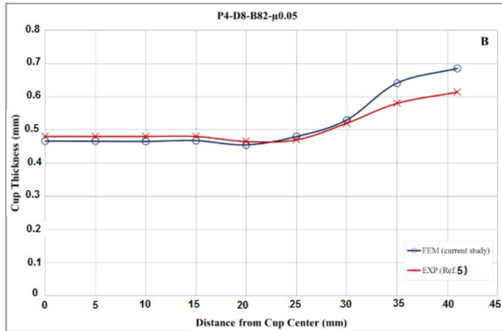
Fig.10-B: Thickness distribution for blank dia.82 mm with (P4-D8) mm.
