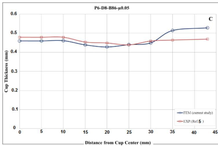
Fig.11-C: Thickness distribution for blank dia.86 mm with (P6-D8) mm.
