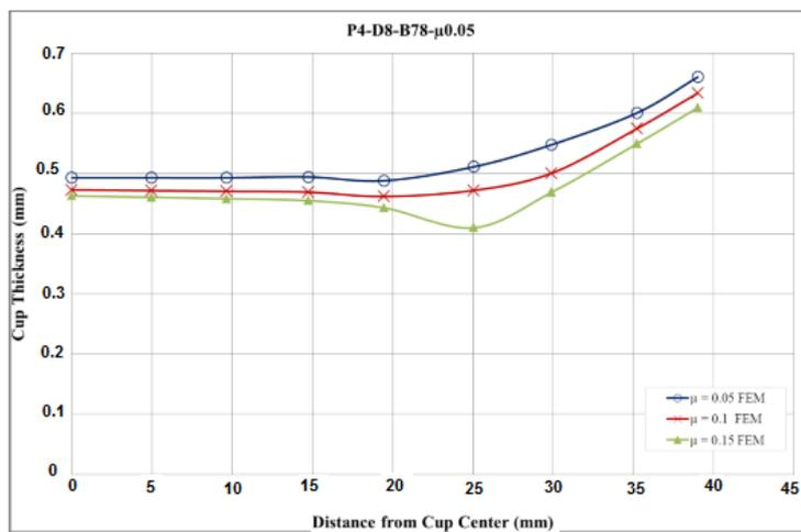
Fig.12 Effect of friction on cup thickness.
