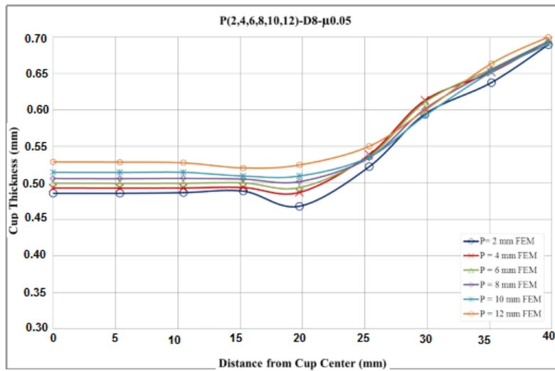
Fig.15 Effect of punch profile radius on thickness distribution.
