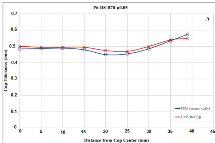
Fig.11-A: Thickness distribution for blank dia.78 mm with (P6-D8) mm.
