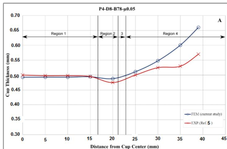
Fig.10-A: Thickness distribution for blank dia.78 mm with (P4-D8) mm.
