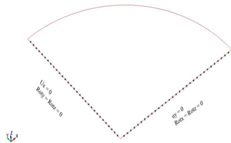
Fig.7 symmetry boundary conditions on blank edges
