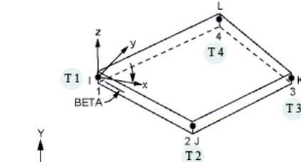
Fig.5 Shell163 geometry[8].
