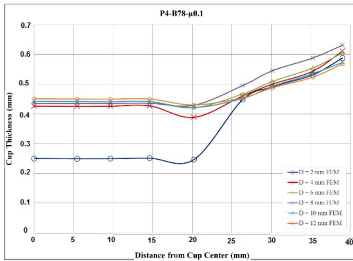
Fig.14 Effect of die profile radius on thickness distribution.
