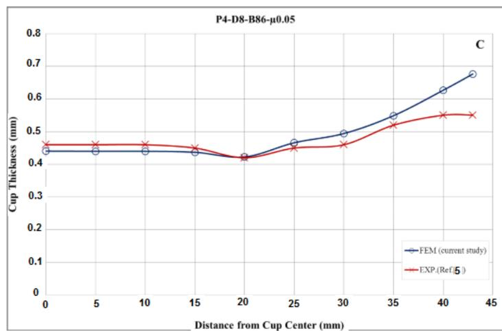
Fig.10-C: Thickness distribution for blank dia.86 mm with (P4-D8) mm.
