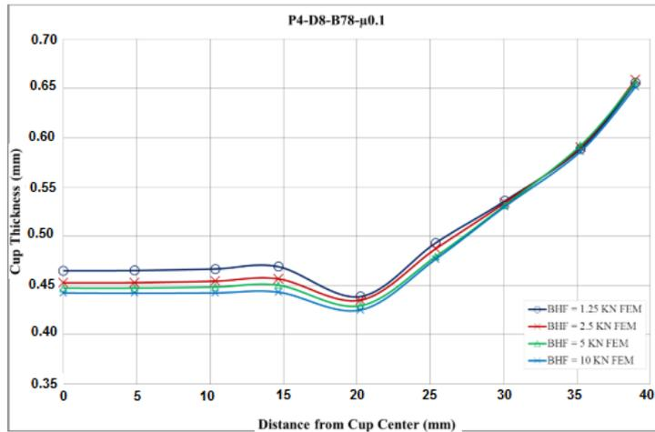
Fig.13 Effect of BHF on thickness distribution
