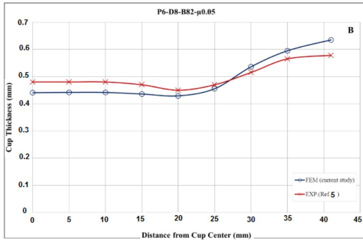
Fig.11-B: Thickness distribution for blank dia.82 mm with (P6-D8) mm.
