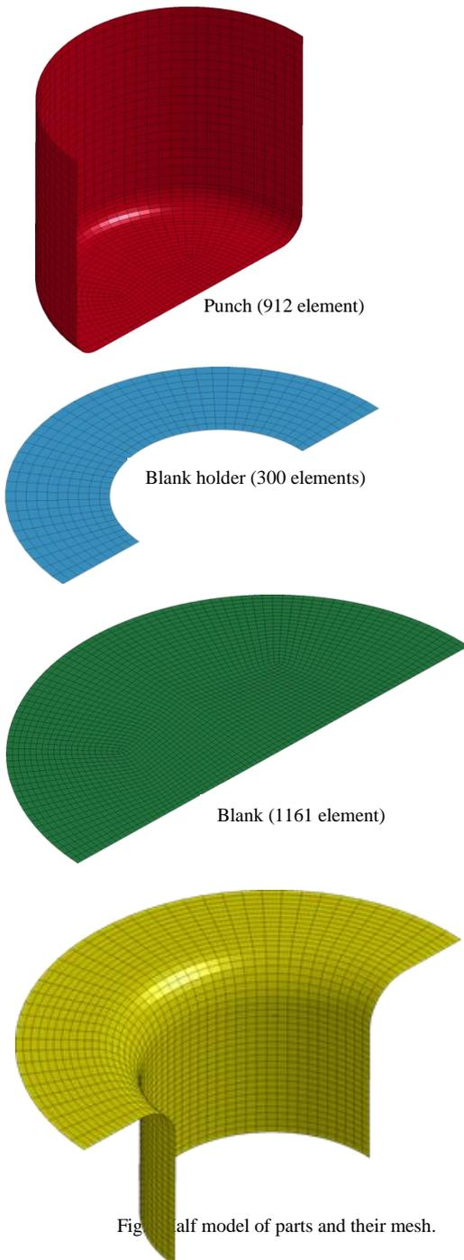
Fig.6 half model of parts and their mesh.
