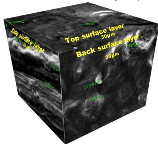
Fig. 4 Cubic body of SEM for 5052 roll wheel side ribbon, transverse side, and airside ribbon produced by RSP with OD of 2.5 mm and G of 2.5 mm at MT of 1000 °C.
