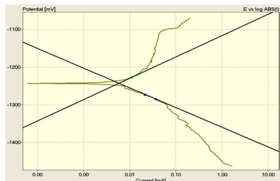
Fig. 14 CorrosionTafel plot for rapid solidified ribbons type 5083 produced by RSP through OD of 2.5 mm, G of 2 mm and MT of 850 °C.
