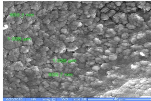
Fig. 8 SEM for 5083 ribbon produced by RSP through OD of 2.5 mm, G of 2 mm and MT of 850 °C.
