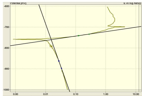
Fig. 13 CorrosionTafel plot for 5083 as received
