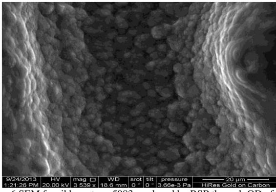
Fig. 6 SEM for ribbons type 5083 produced by RSP through OD of 2.5 mm, G of 2 mm and MT of 850 °C.
