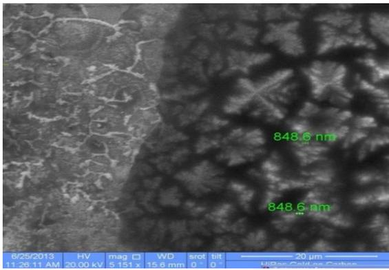
Fig. 7 SEM for 5083 ribbon produced by RSP through OD of 2.5 mm, G of 5 mm and MT of 850 °C.
