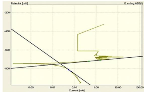
Fig. 11 CorrosionTafel plot for alloy type 5052 as received
