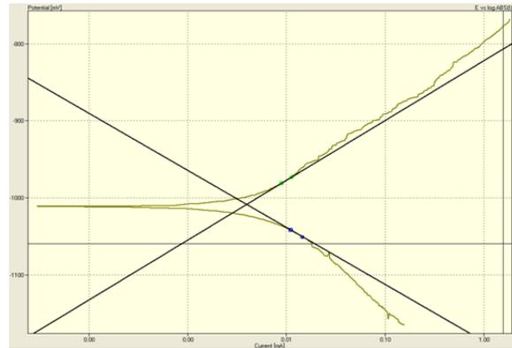
Fig. 12 CorrosionTafel plot for rapid solidified ribbons type 5052 produced by RSP through OD of 3.5 mm, G of 2 mm and MT of 750 °C.
