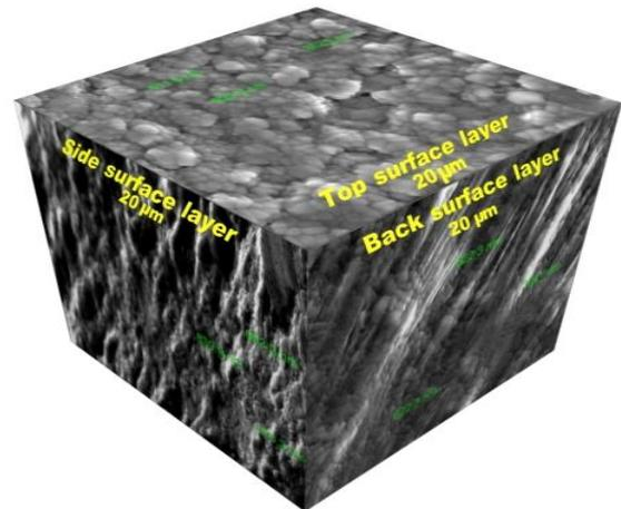
Fig. 9 Cubic body of SEM for 5083 roll wheel side ribbon, transverse side, and airside ribbon produced by RSP through OD of 2.5 mm, G of 2 mm and MT of 850 °C.
