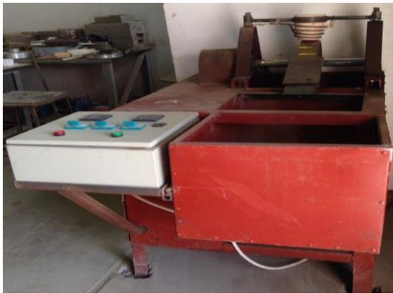
Fig. 1 Single roll melt spinning machine
