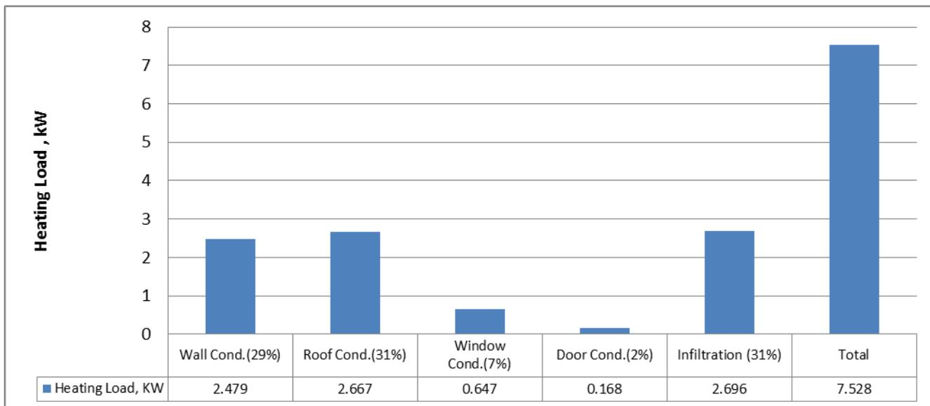
Fig. 4 Building peak heating load components for the base house (Dec 30 6AM).
