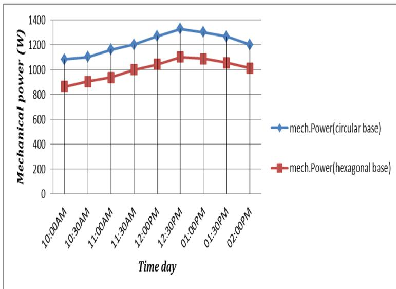
Fig.11 The mechanical power of chimney and time day at 15 January
