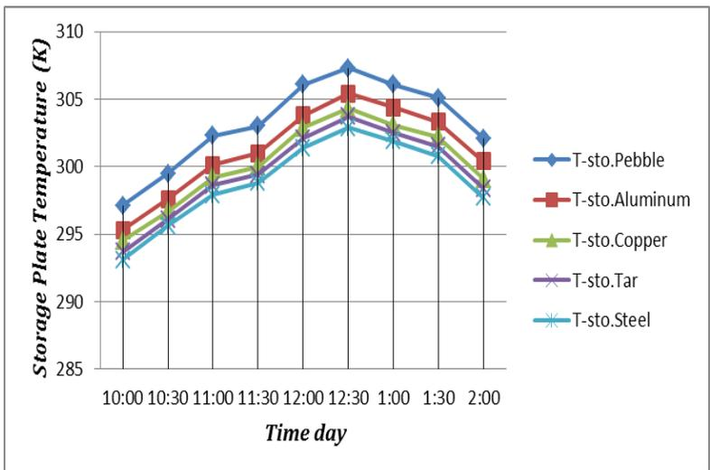
Fig. 5 The temperature of storage plate and time day at 15 January
