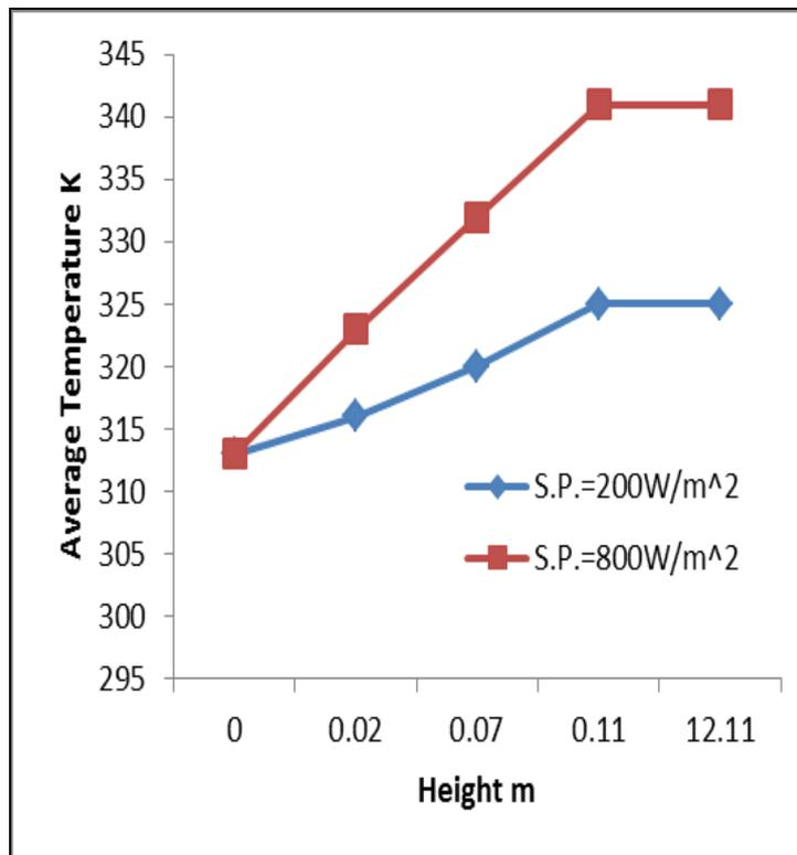
Fig. 17 The average temperature (K) of system for both cases of beam solar flux
