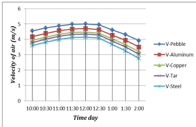
Fig. 7 The velocity of air in chimney and time day at 14 March
