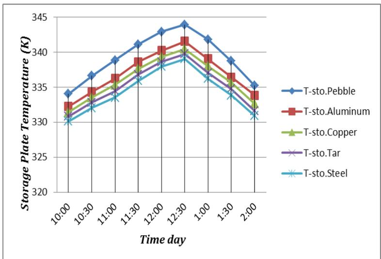
Fig. 3 The temperature of storage plate and time day at 1 July
