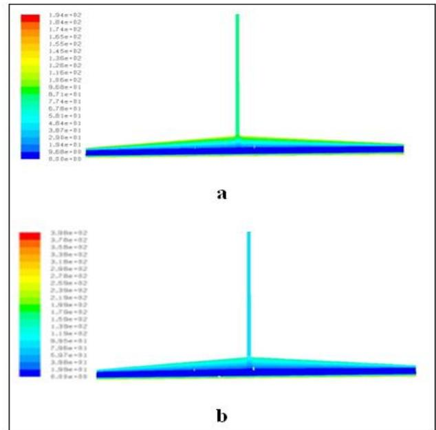
Fig. 14 Solar heat flux (W/m<sup>2</sup>) for two cases of beam solar arrays a- at 200W/m<sup>2</sup>, b- at 800W/m<sup>2</sup>
