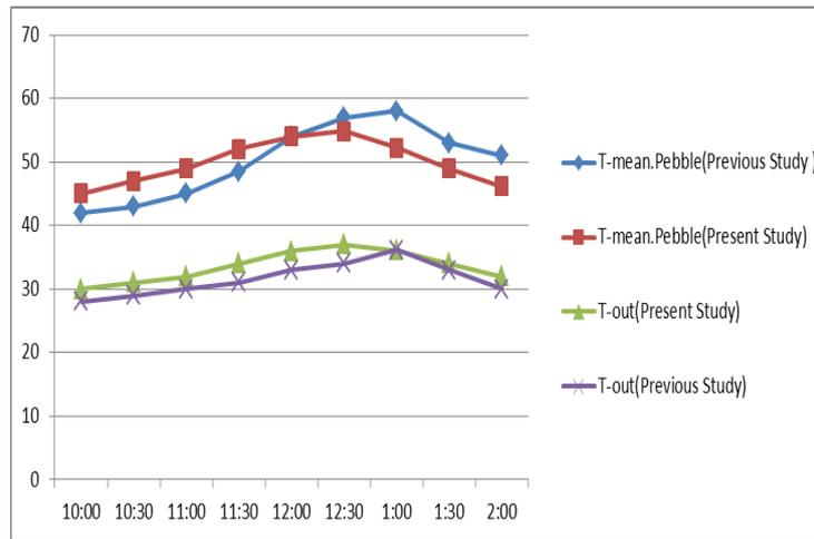
Fig.12 The temperature comparison of air in centroid of solar collector and time day with storage plate of black pebble at 14 March for present study with 15 September for previous study [8]
