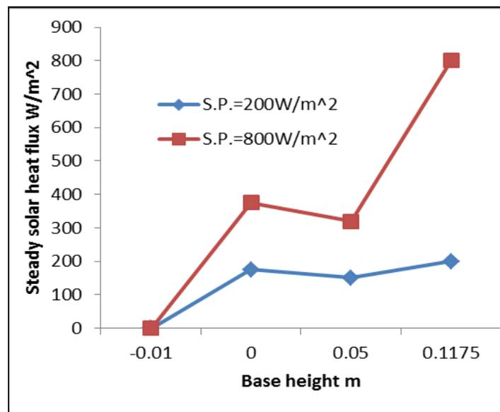
Fig. 15 The steady solar heat flux of system for both cases of beam solar flux(the coordinates according to Fig.1)
