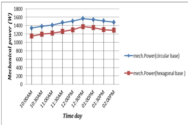
Fig.10 The mechanical power of chimney and time day at 14 March
