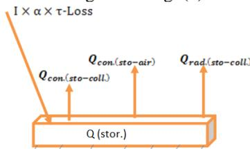
Fig. 2 thermal analysis of storage plate
