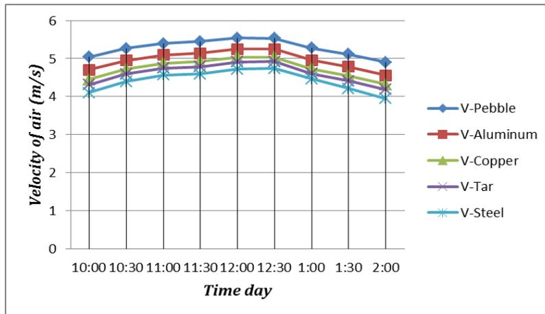
Fig. 6 The velocity of air in chimney and time day at 1 July
