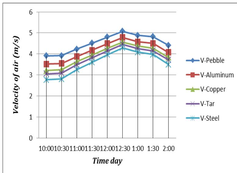
Fig.8 The velocity of air in chimney and time day at 15 January
