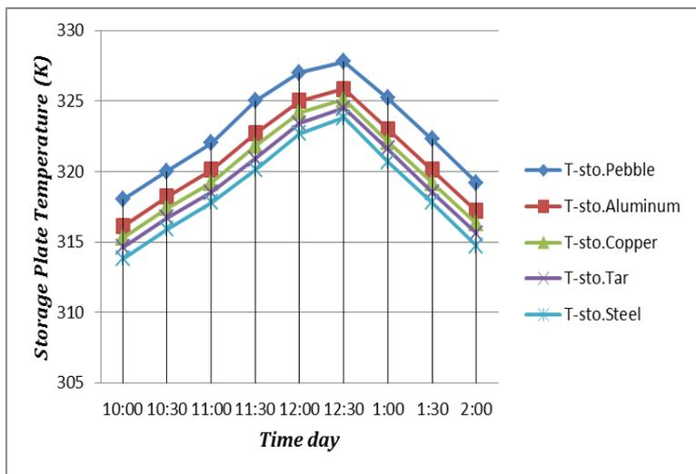
Fig. 4 The temperature of storage plate and time day at 14 March
