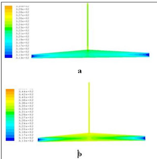
Fig. 13 Temperature contour for different solar flux a- 200W/m<sup>2</sup>, b- 800W/m<sup>2</sup>
