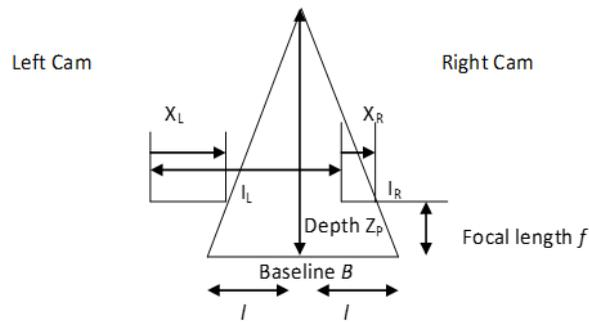
Figure 4: Demonstration of stereo image system
