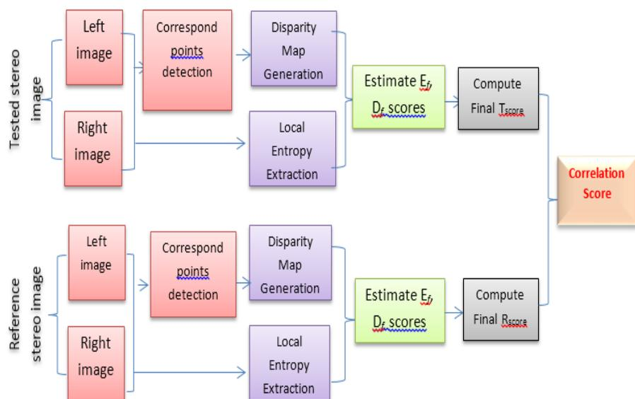
Figure 2: The framework of ED-QA objective quality model
