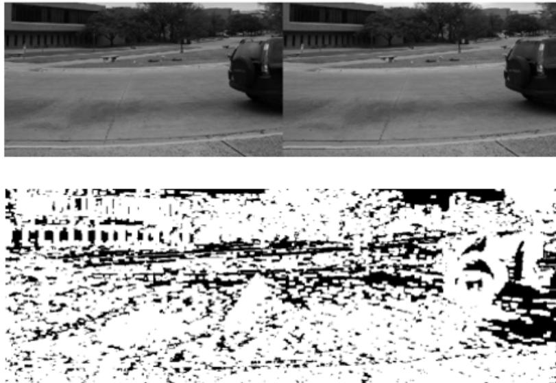
**Figure 5:** Sample of stereoscopic image and its disparity map image: the top image is the original stereo pair image, the bottom image is the disparity map for the original image.
