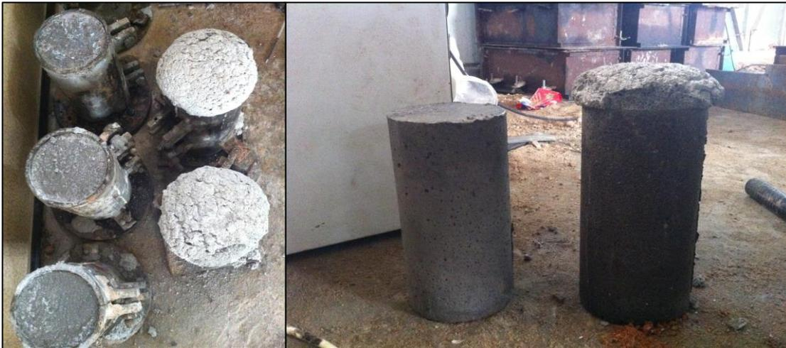
**Figure 4** Swelling of specimens after short period of mixing and casting
