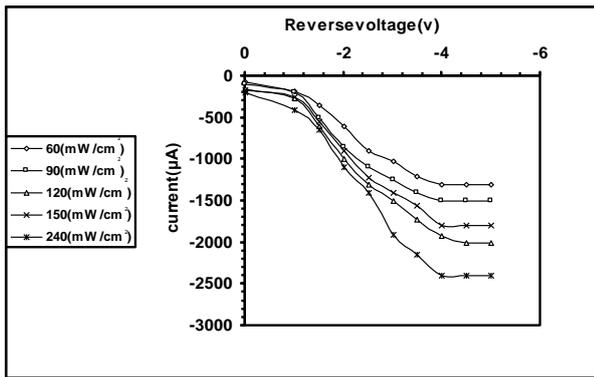
**Fig.(4) : (I-V) characteristics under different power density illumination.**
