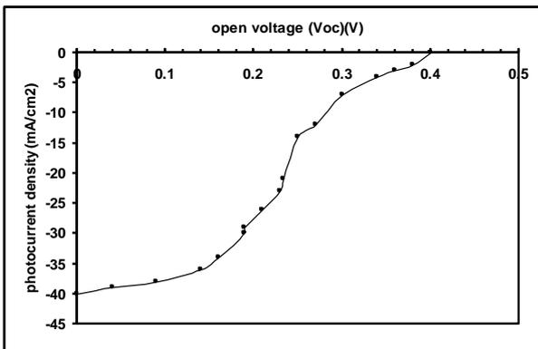
**Fig.(5) : The photovoltaic performance of the cell under condition AM1.**
