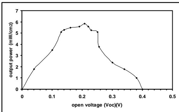
**Fig.(6) : The output power generated by the cell.**
