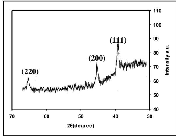
**Fig.(1) : XRD spectra of CdO film on glass substrate .**
