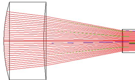
Fig.(1) : Two lenses for Beam Expander.
