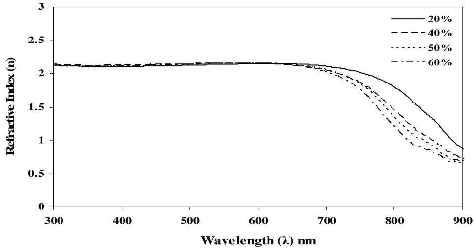
Fig. (4) Refractive index versus wavelength for different percentage of Al<sub>2</sub>O<sub>3</sub>.
