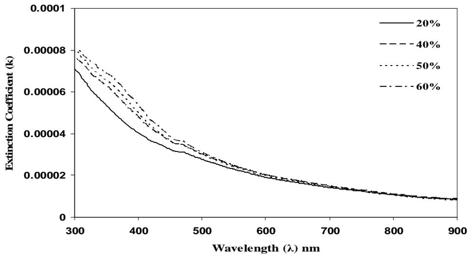
Fig. (5) Extinction coefficient versus wavelength for different percentage of Al<sub>2</sub>O<sub>3</sub>.
